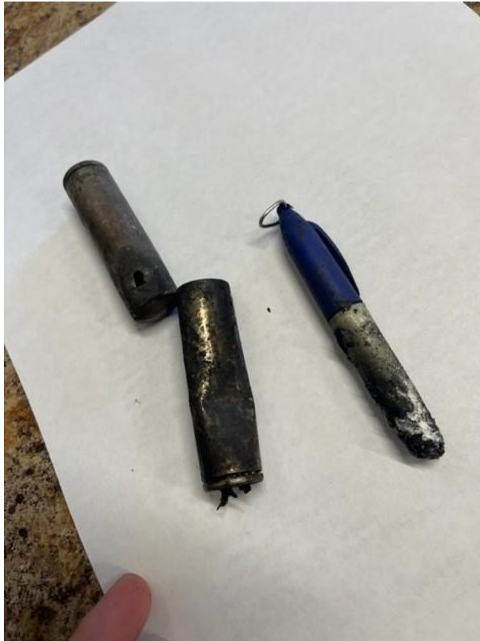
Photo 1 – Burnt Batteries and Pen, Photo provided by Air Evac LifeTeam
