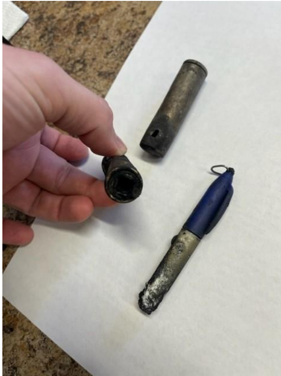
Photo 2 – Burnt Battery, Photo provided by Air Evac LifeTeam
