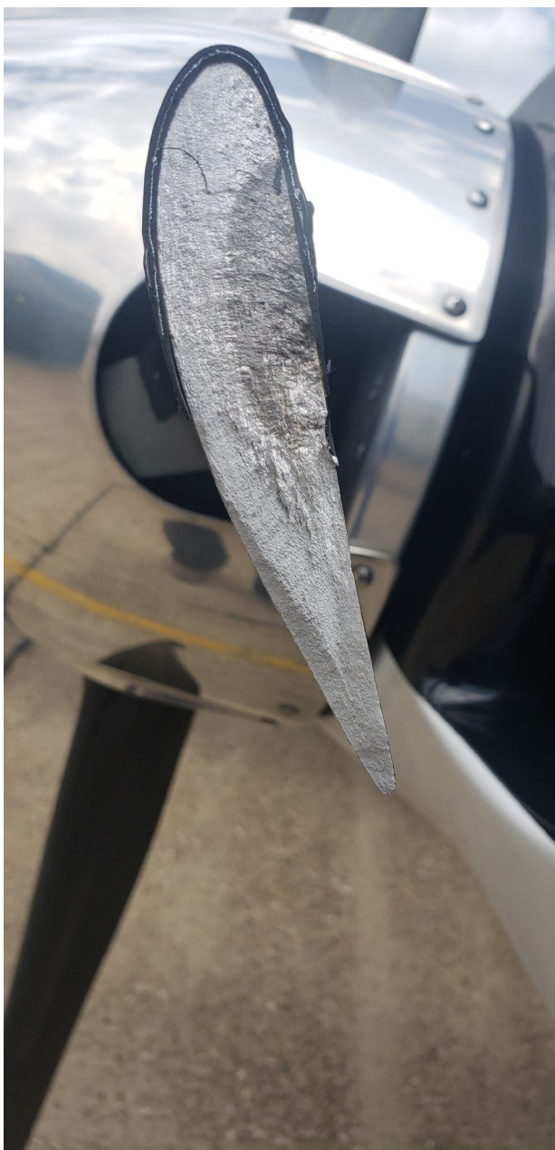
Photo 3 – View of the fractured left side propeller blade after the airplane landed (courtesy of the pilot).
