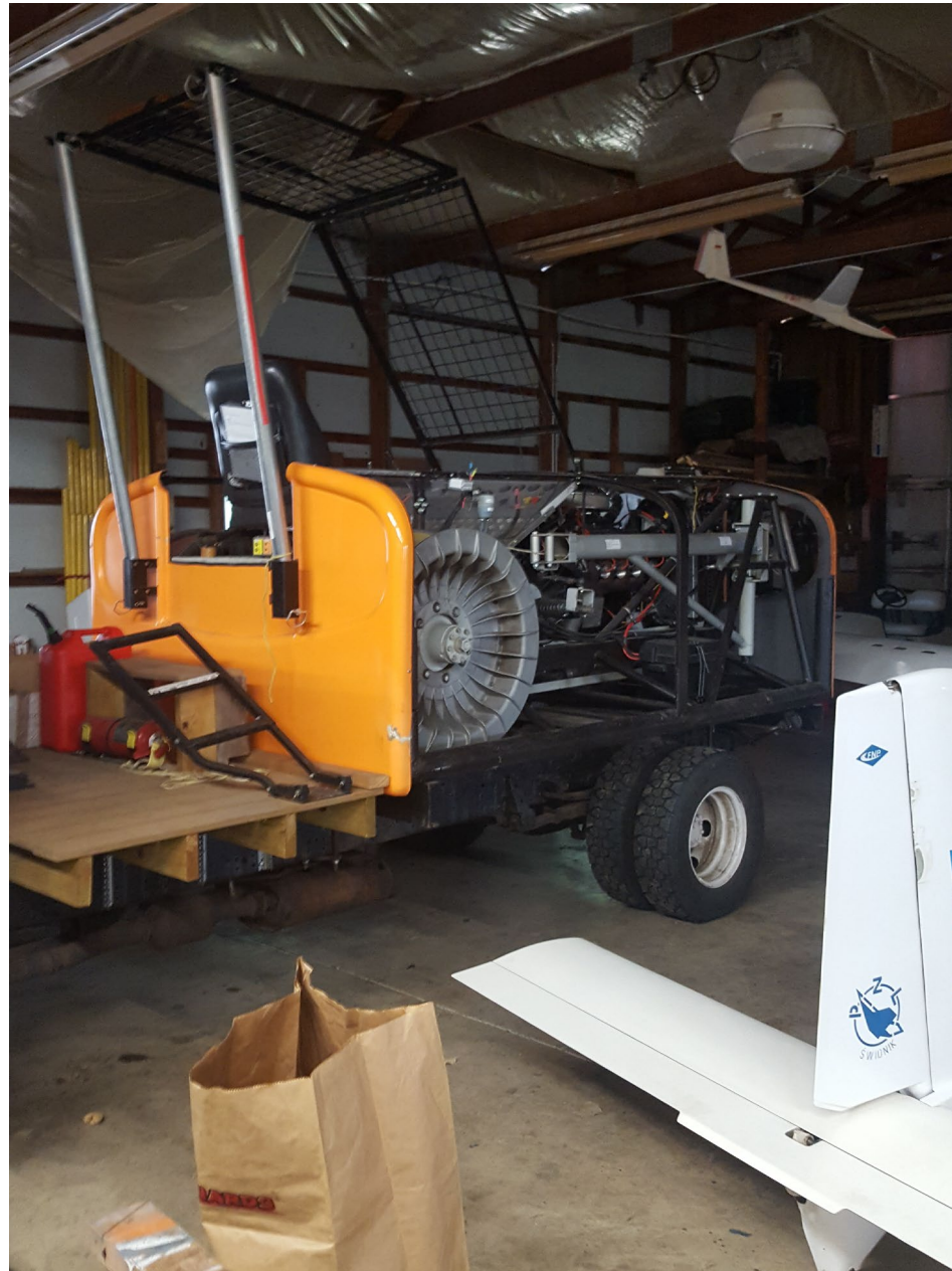
Photo 1 – View of the ground winch system (courtesy of the flight instructor).
