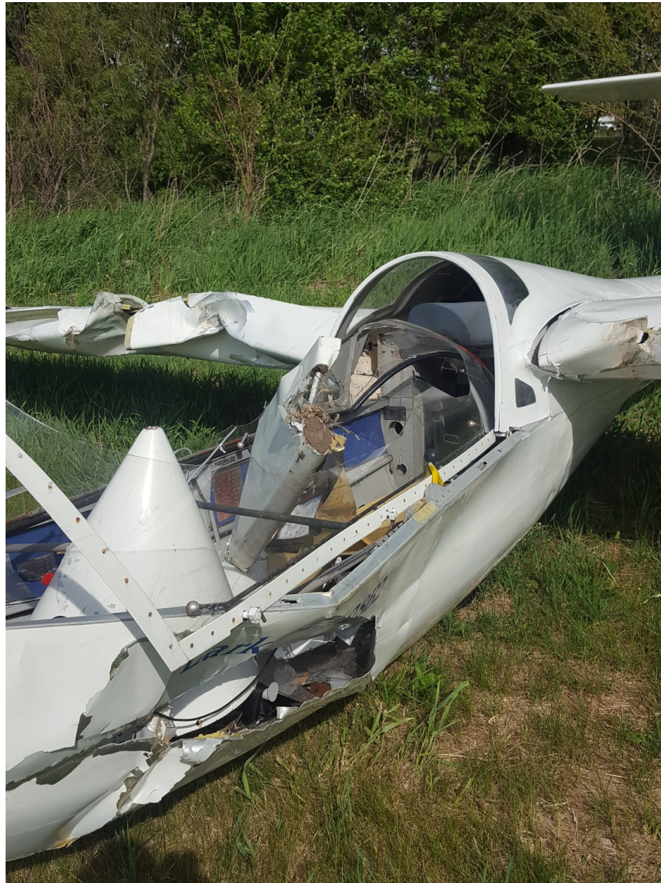
Photo 4 – View of the substantial damage sustained to the fuselage and both wings (courtesy of the flight instructor).
