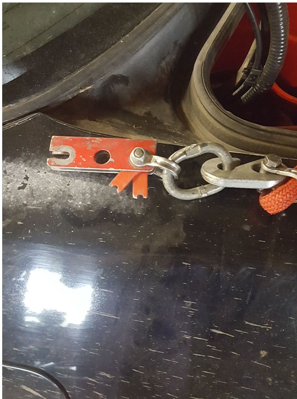
Photo 2 – View of the broken weak link/safety link (courtesy of the flight instructor).
