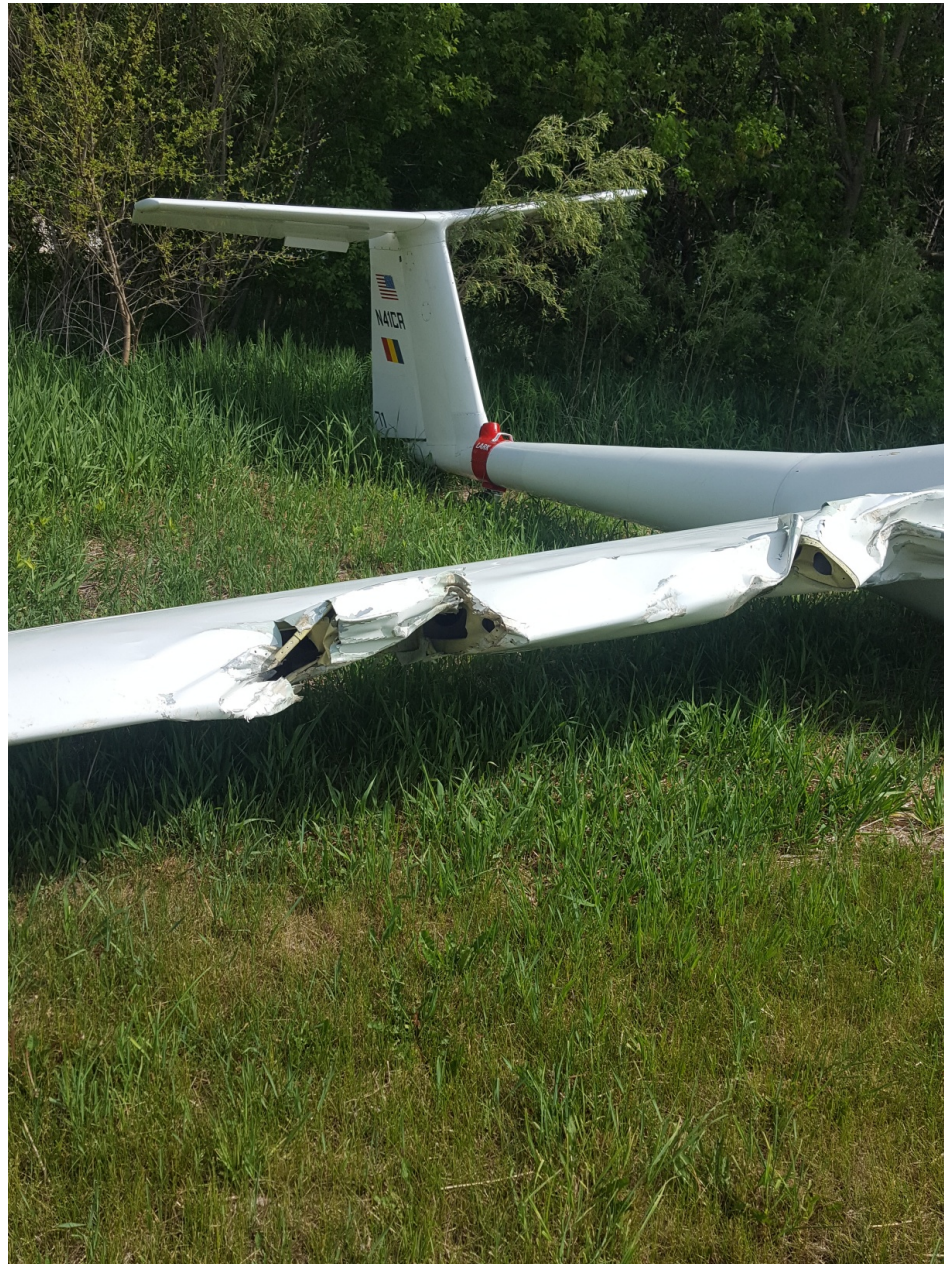
Photo 5 – View of the substantial damage sustained to the right wing (courtesy of the flight instructor).
