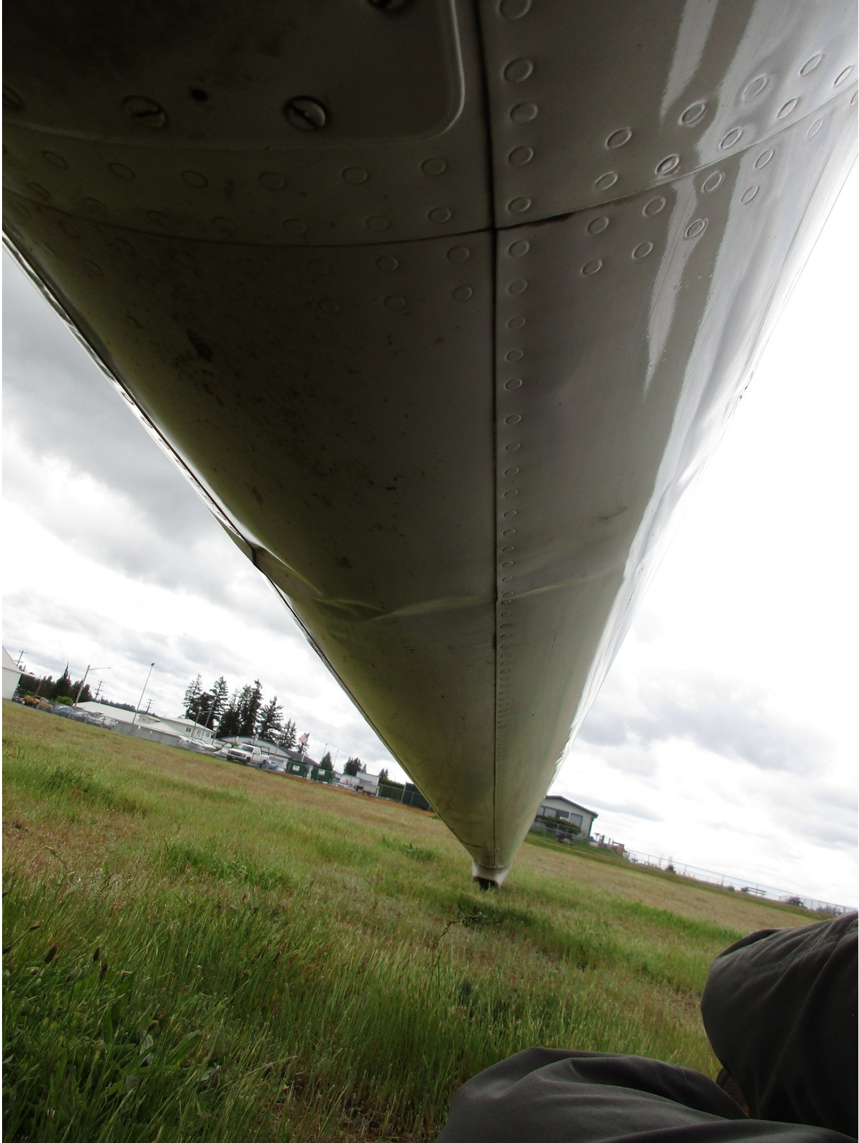
Photo 2: Damage to empennage (FAA)
