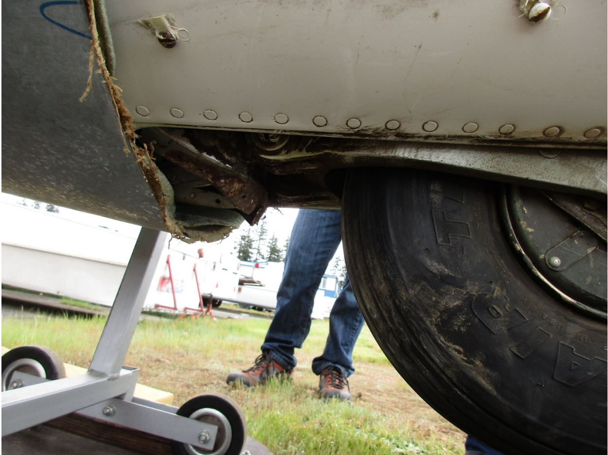
Photo 3: Damage to fuselage and landing gear (FAA)
