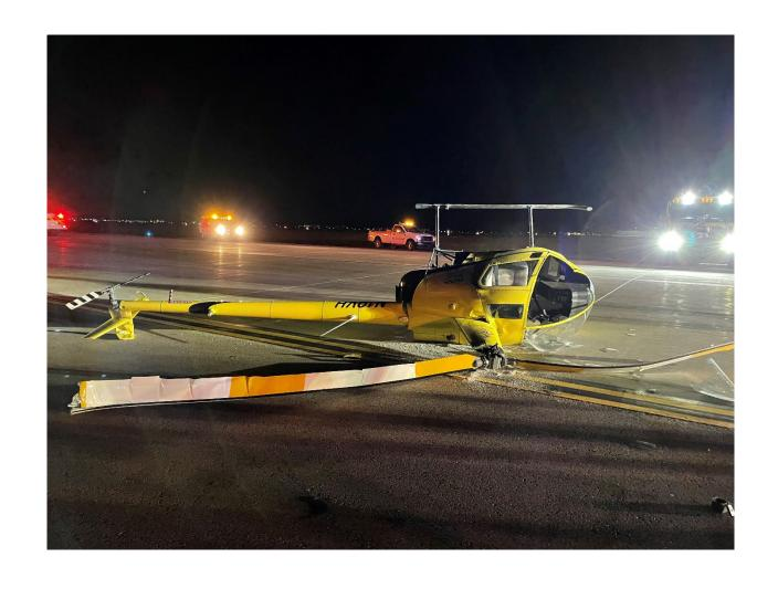
Photo 1 – View of damage to the horizontal stabilizer, wind screen, and main rotor system (Courtesy of FAA)
