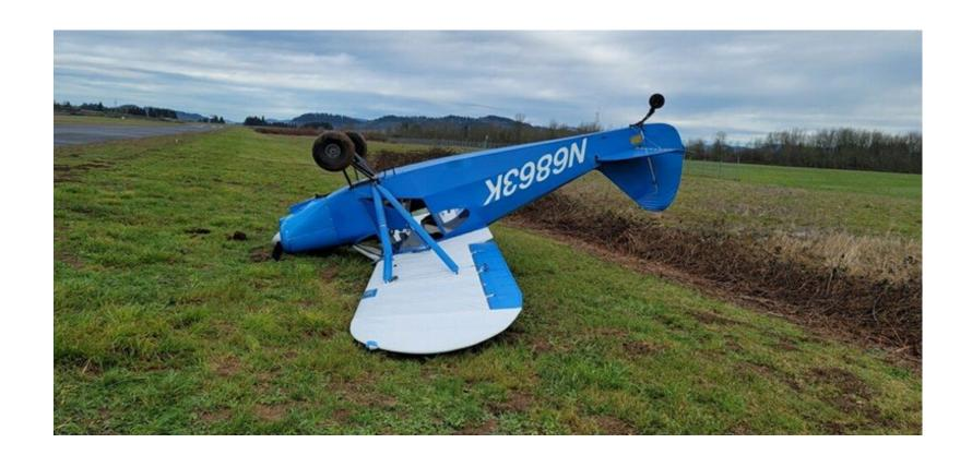
Photo 1 – View of damage to the right wing lift strut and rudder (Courtesy of Operator)
