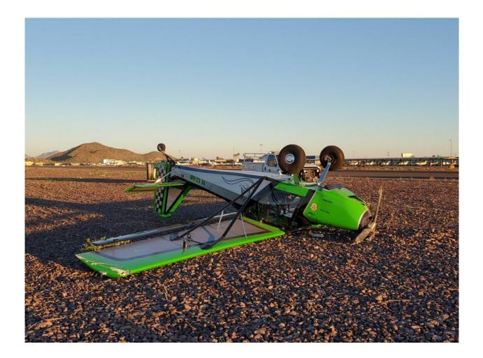
Photo 1 – View of damage to the left forward wing lift strut (Courtesy of FAA)
