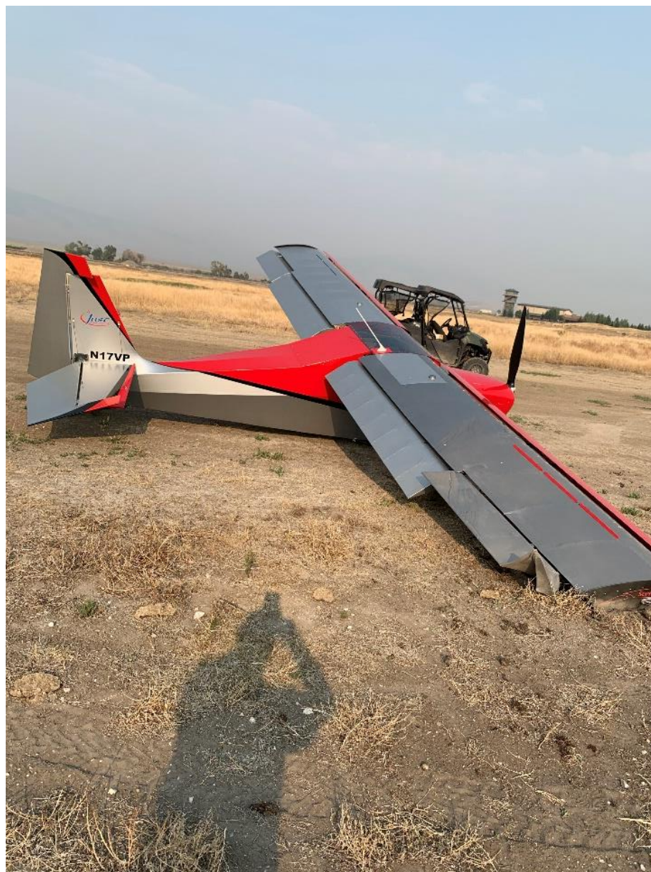
Photo 1 – View of damage to the right wing aileron (Courtesy of the Pilot)
