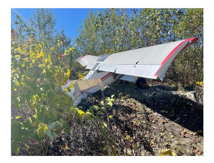
Photo 1 – View of damage to the empennage and the left wing (Courtesy of Operator)
