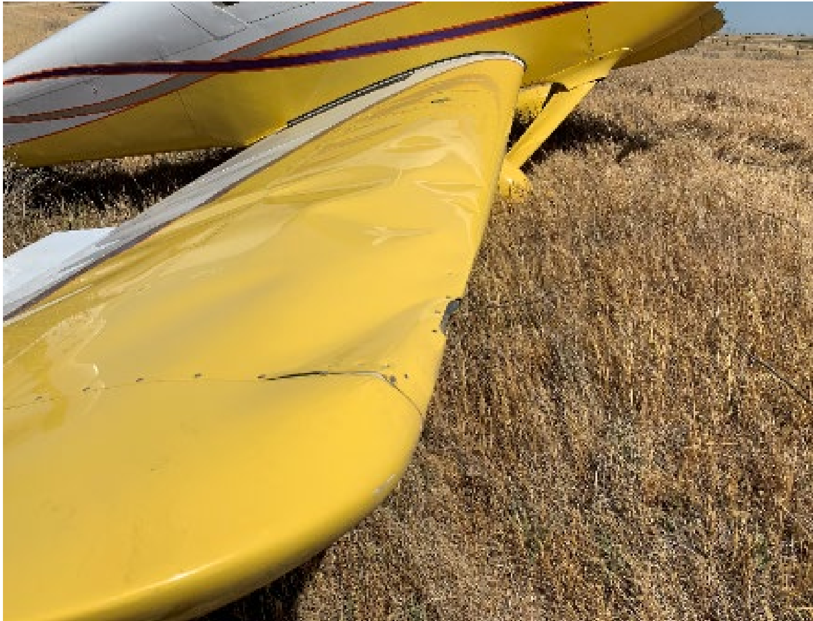
Photo 1 – View of substantial damage the right wing (Courtesy of Pilot)
