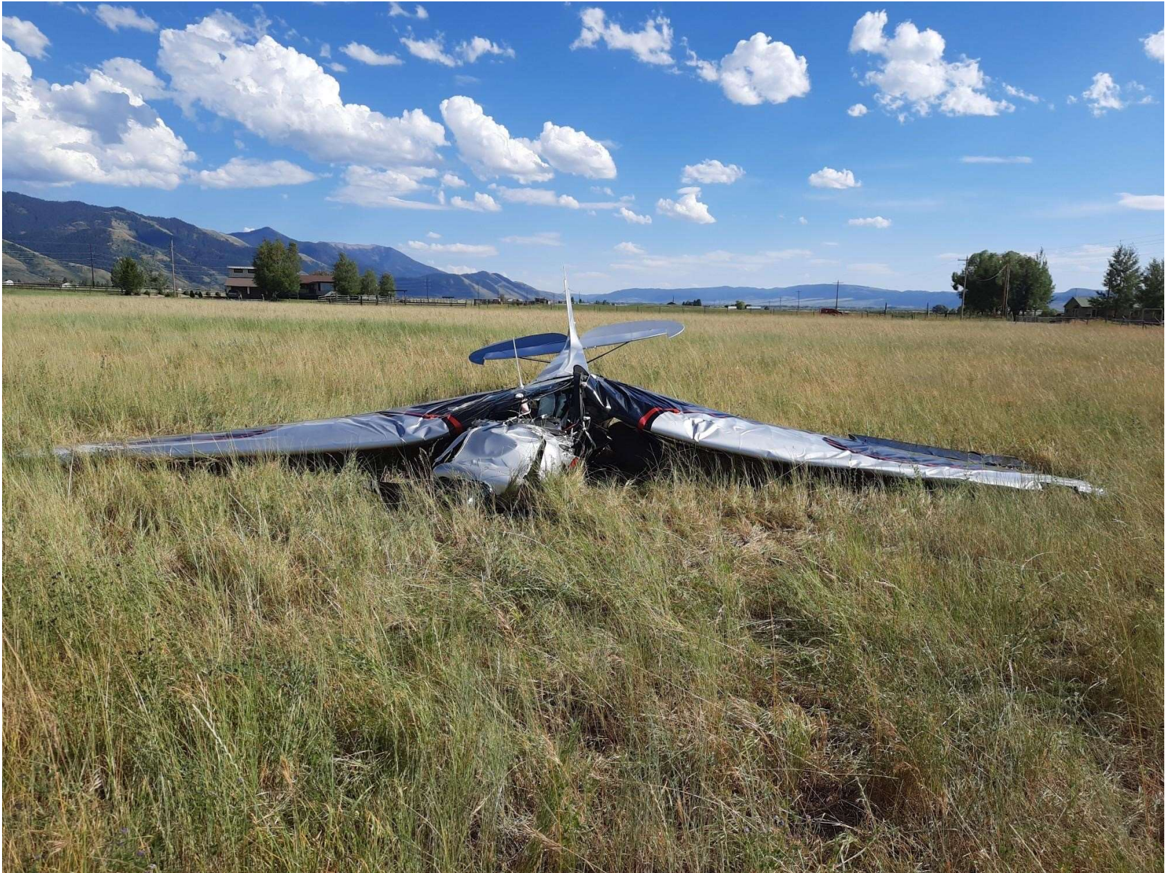
Photo 1 – View of substantial damage to the airplane’s wings and fuselage (Courtesy of FAA)
