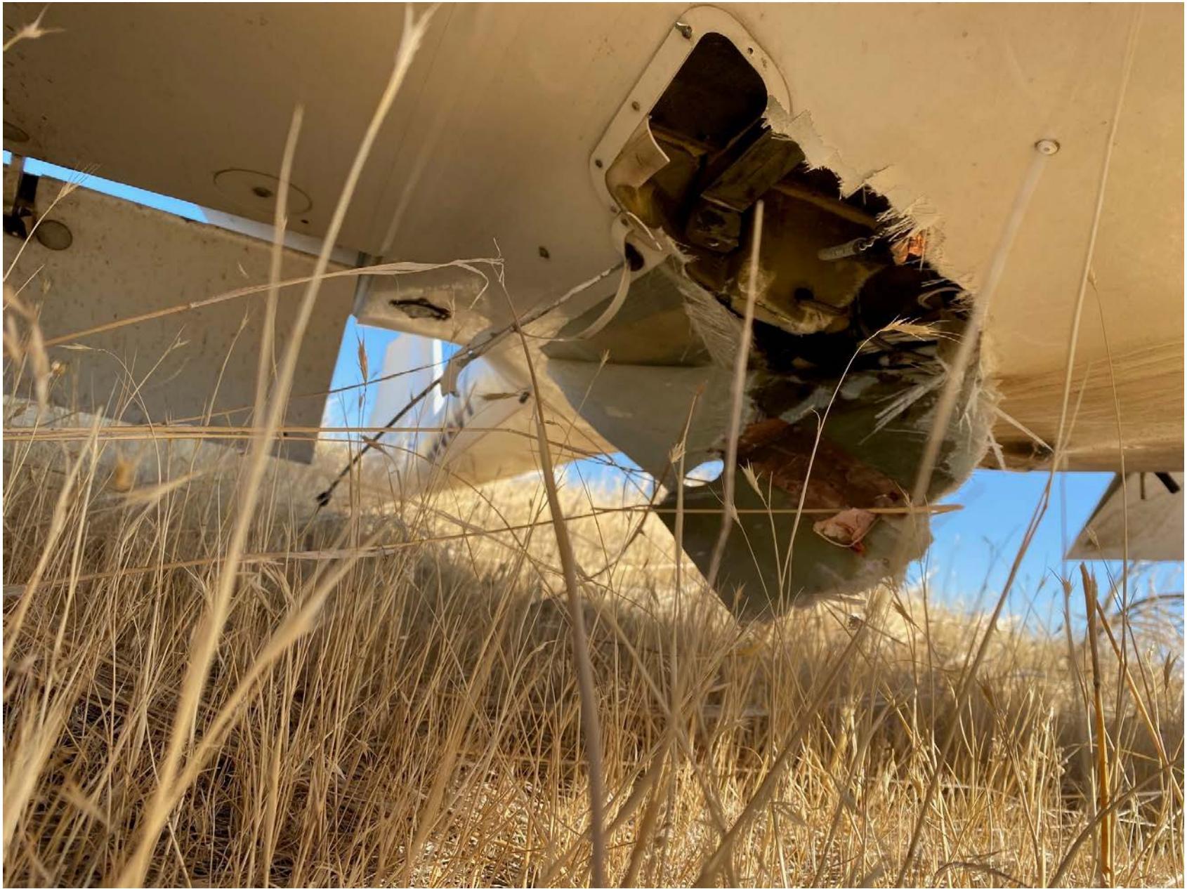
Photo 1 – View of damage to the lower fuselage (Courtesy of Operator)
