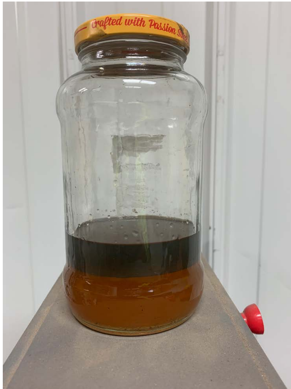
Photo of Fuel Drained from Helicopter's Gascolator
