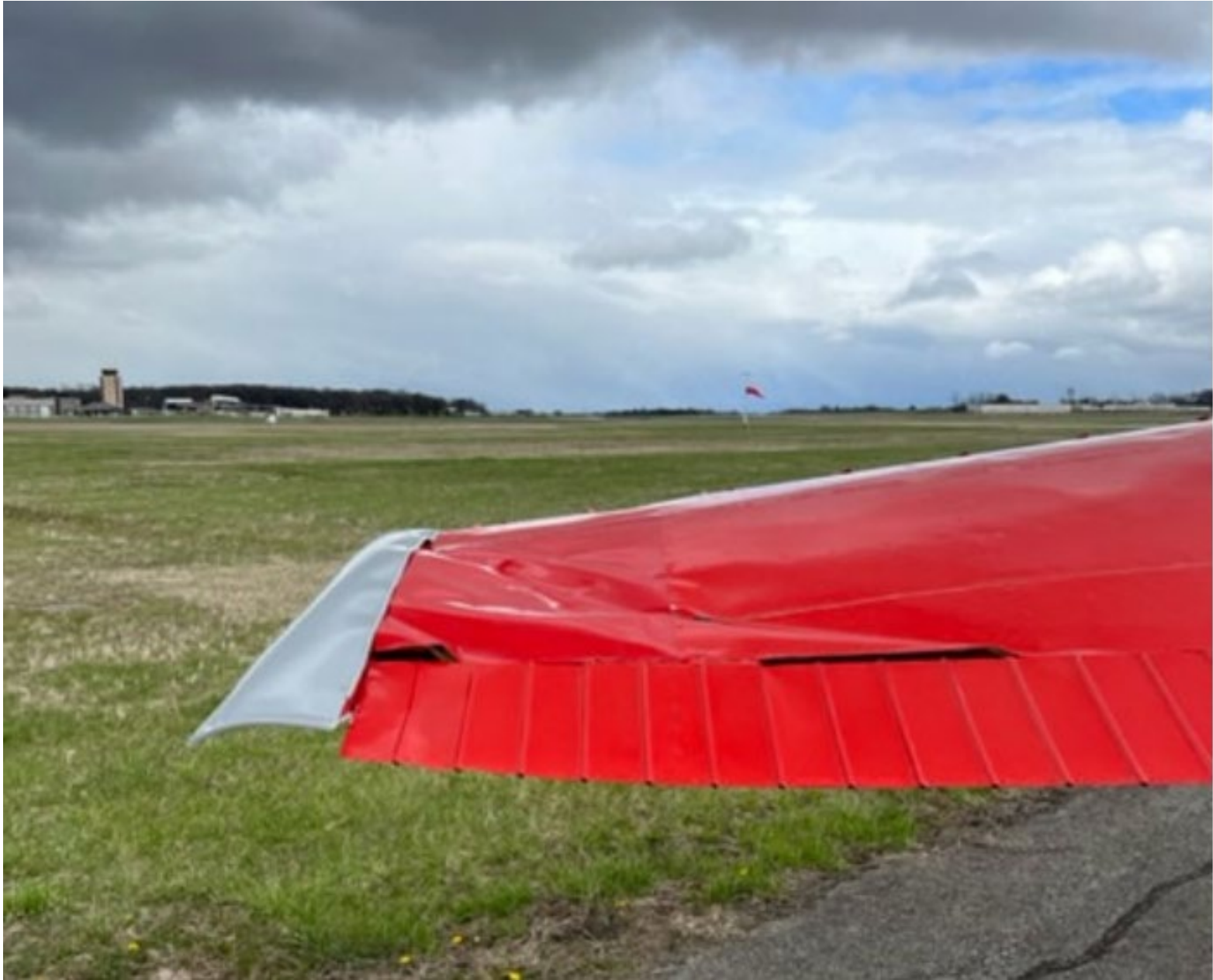
Photo of Damaged Left Wing, Courtesy of Federal Aviation Administration
