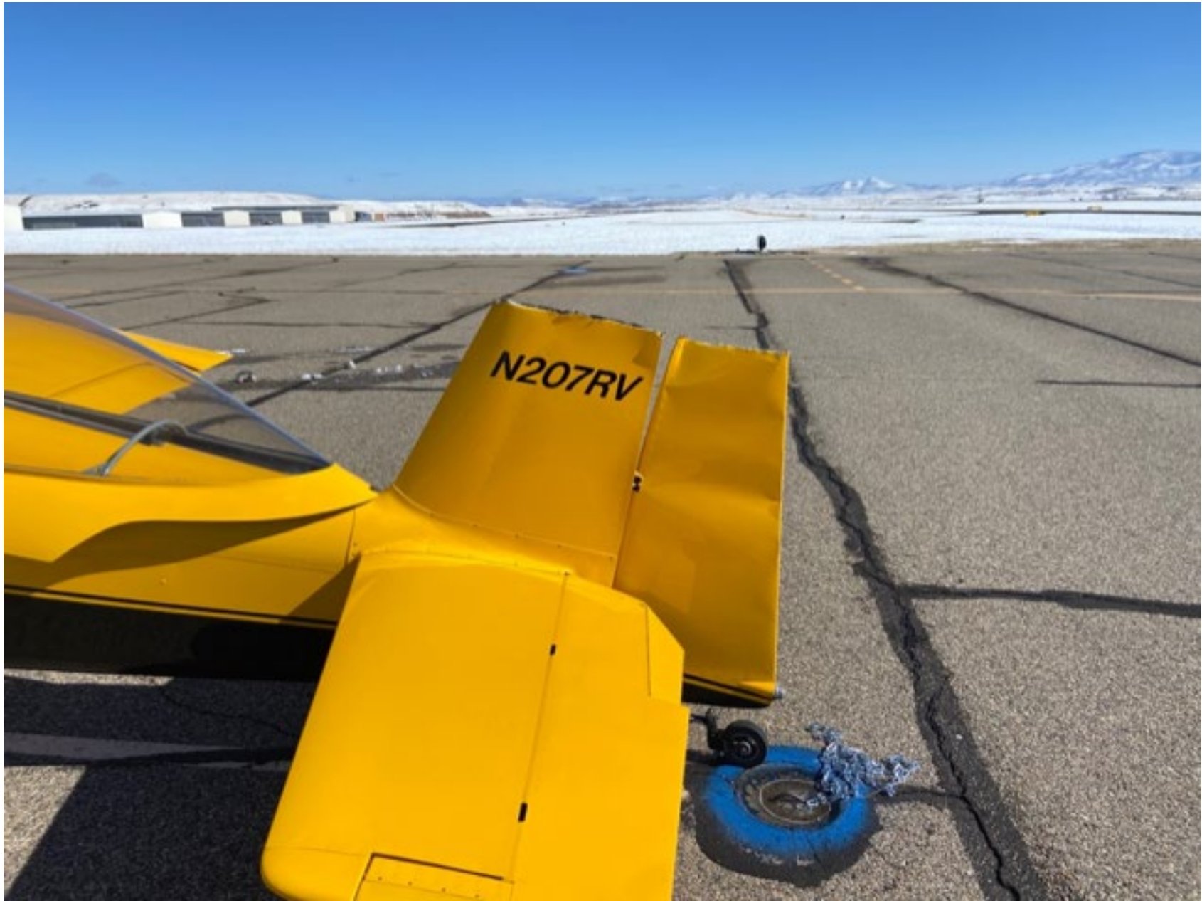
Photo 1 –N207RV, left-side view of damage to the vertical stabilizer and rudder. Photo courtesy of the pilot.
