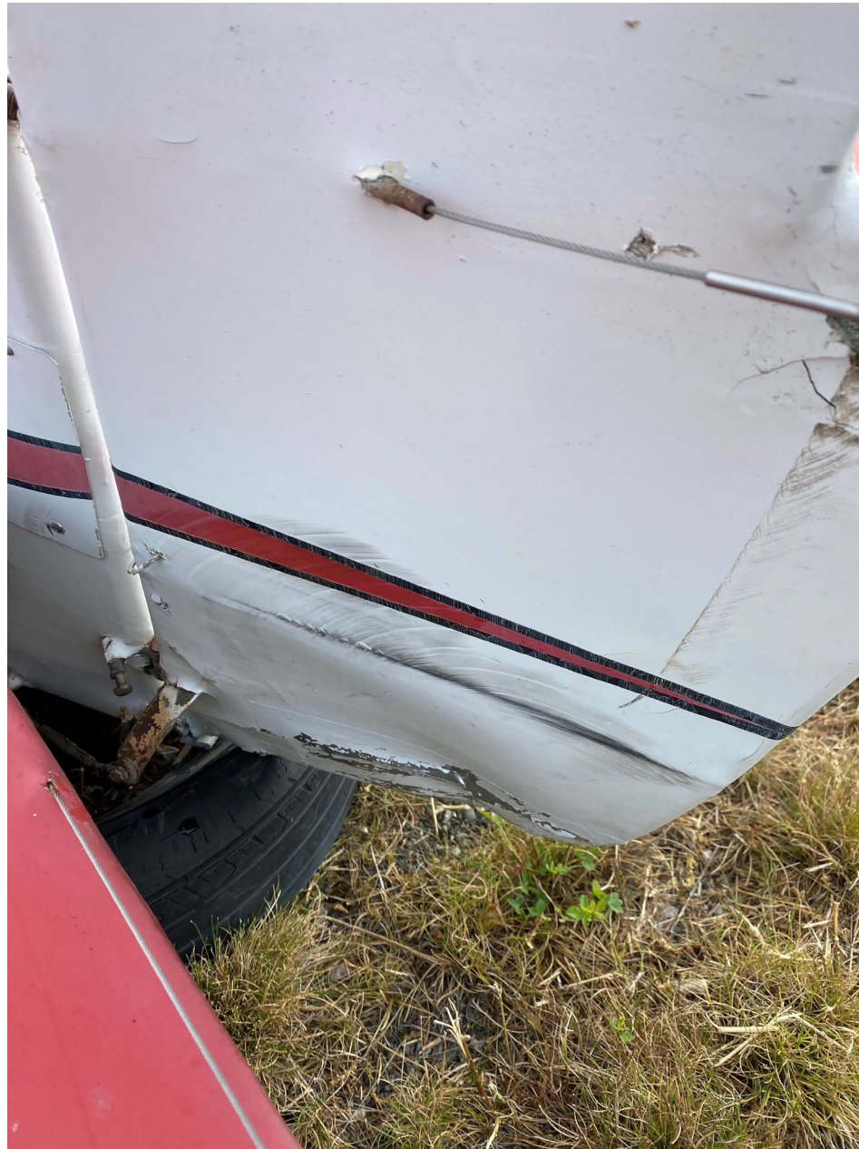
Photo 2 – Accident airplane’s damaged rudder. Photo provided by mechanic.
