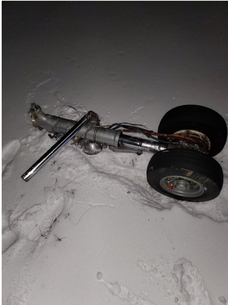
Photo 3 – Main landing gear separated from airplane
