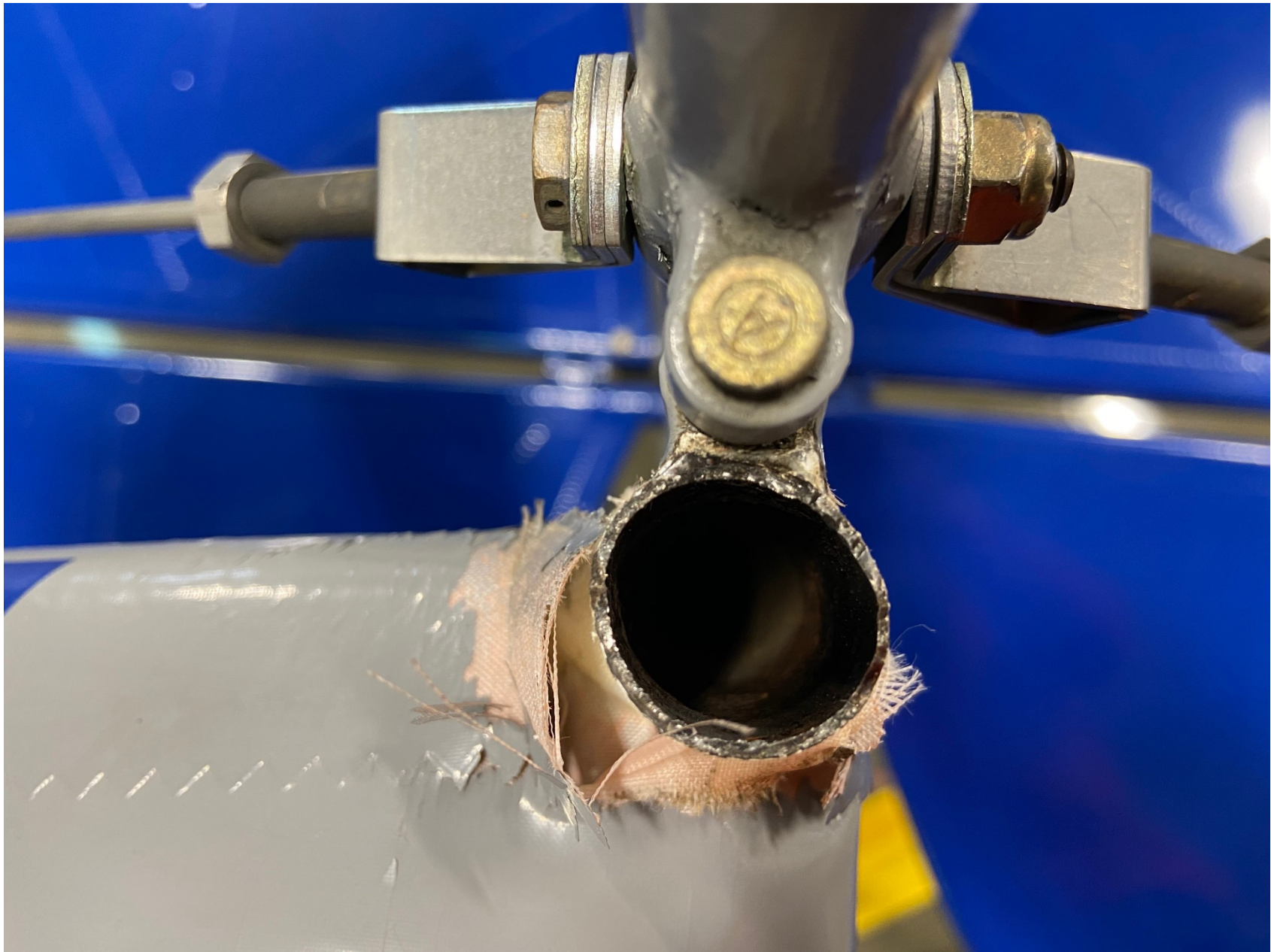
Photo 3 – Accident airplane's fractured rudder post.
