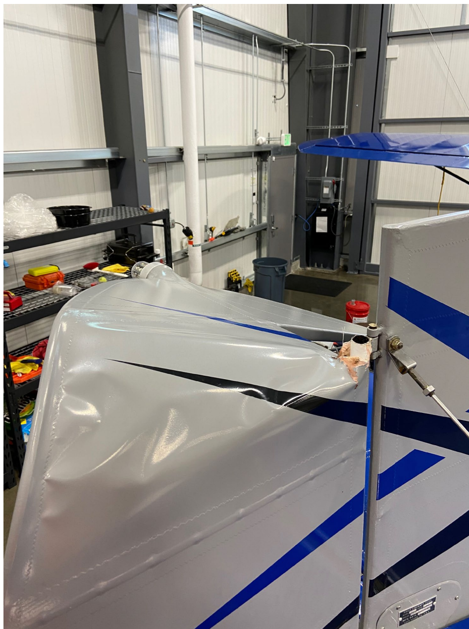
Photo 2 – Accident airplane’s substantially damaged rudder.
