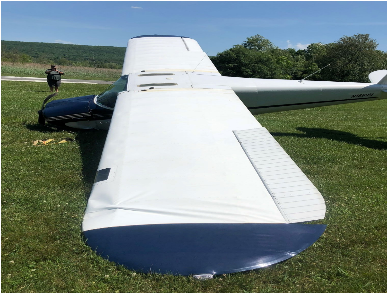
Photo 1 – View of left wing showing buckling damage on outboard section of wing (FAA Photo)
