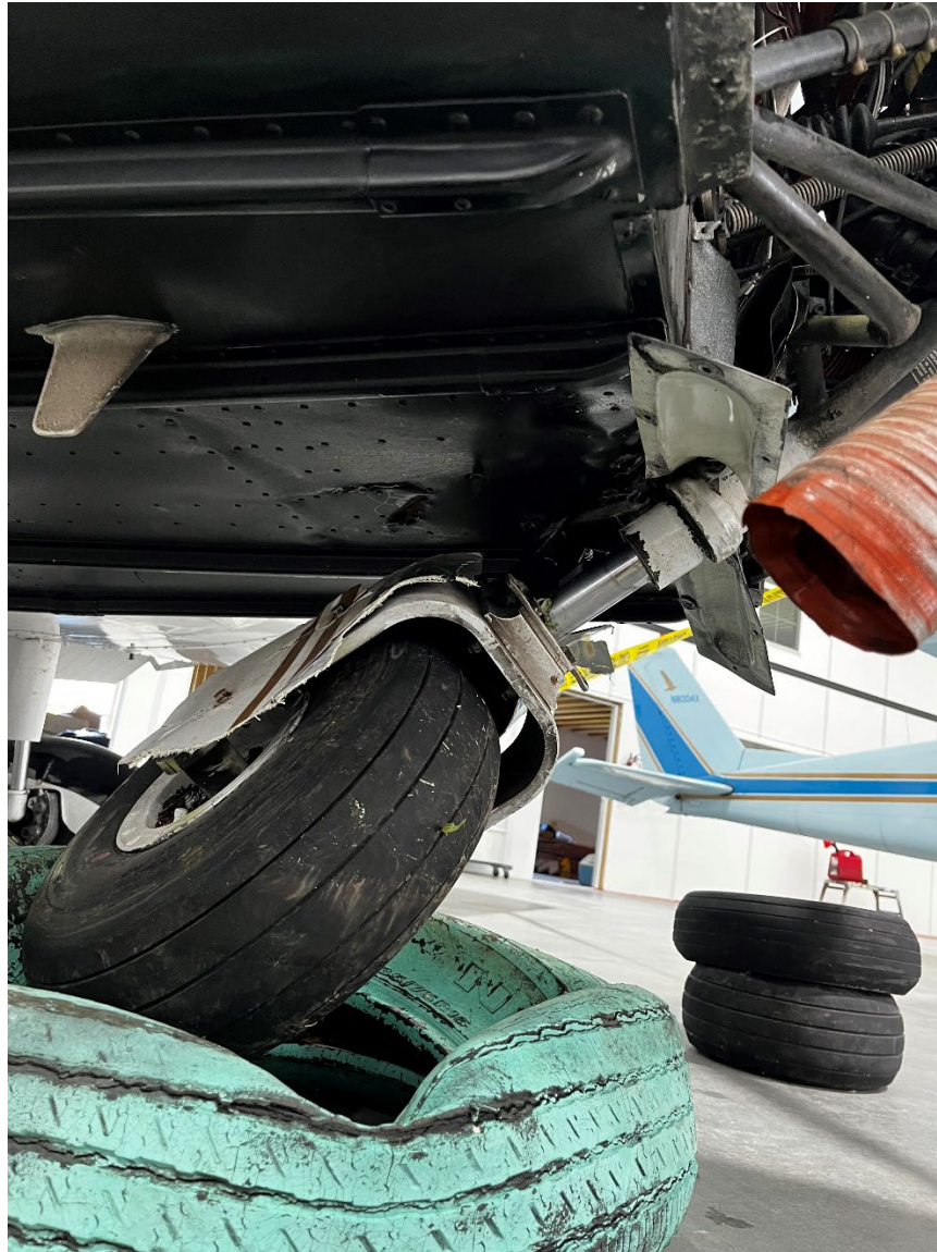
Photograph 2 - Fuselage Damage (Courtesy of Federal Aviation Administration)
