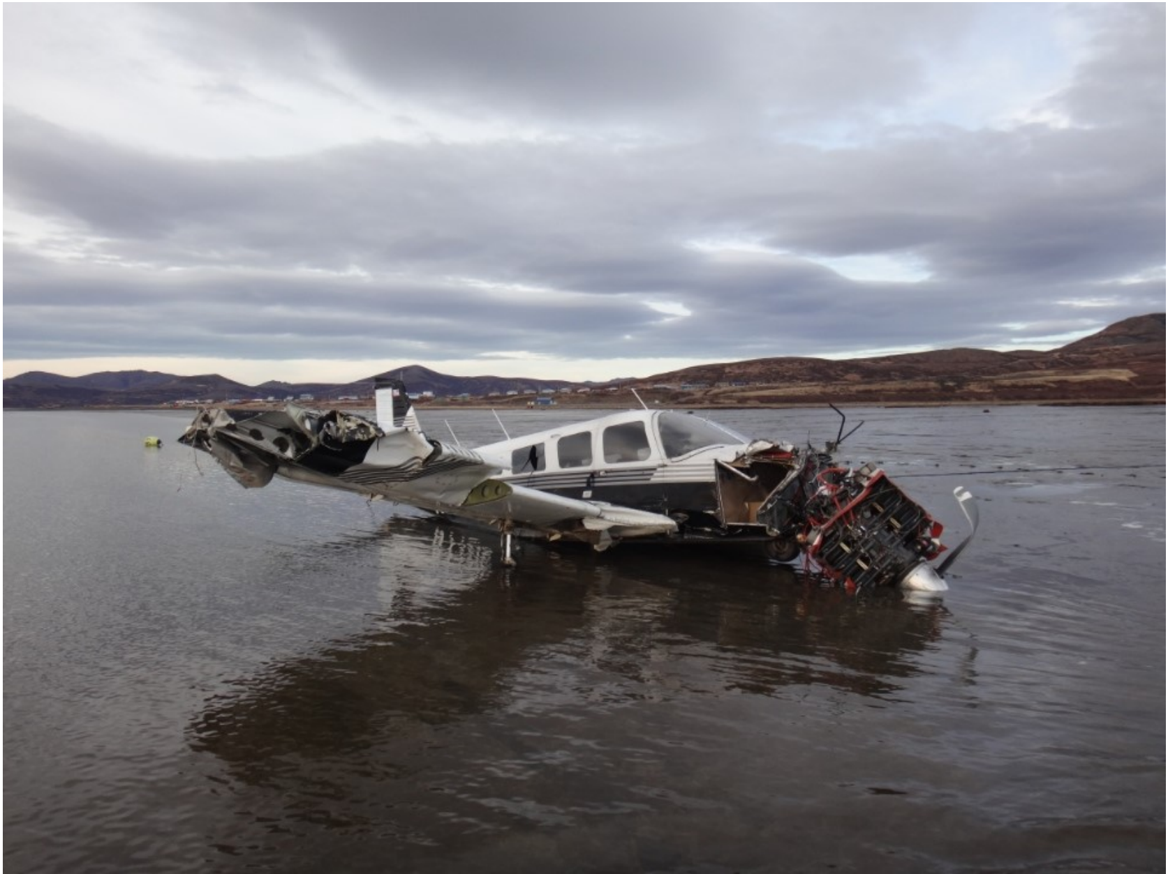
Photo 5 - Wreckage right side with right wing and propeller damage evident. (Source: Yute Commuter Services)
