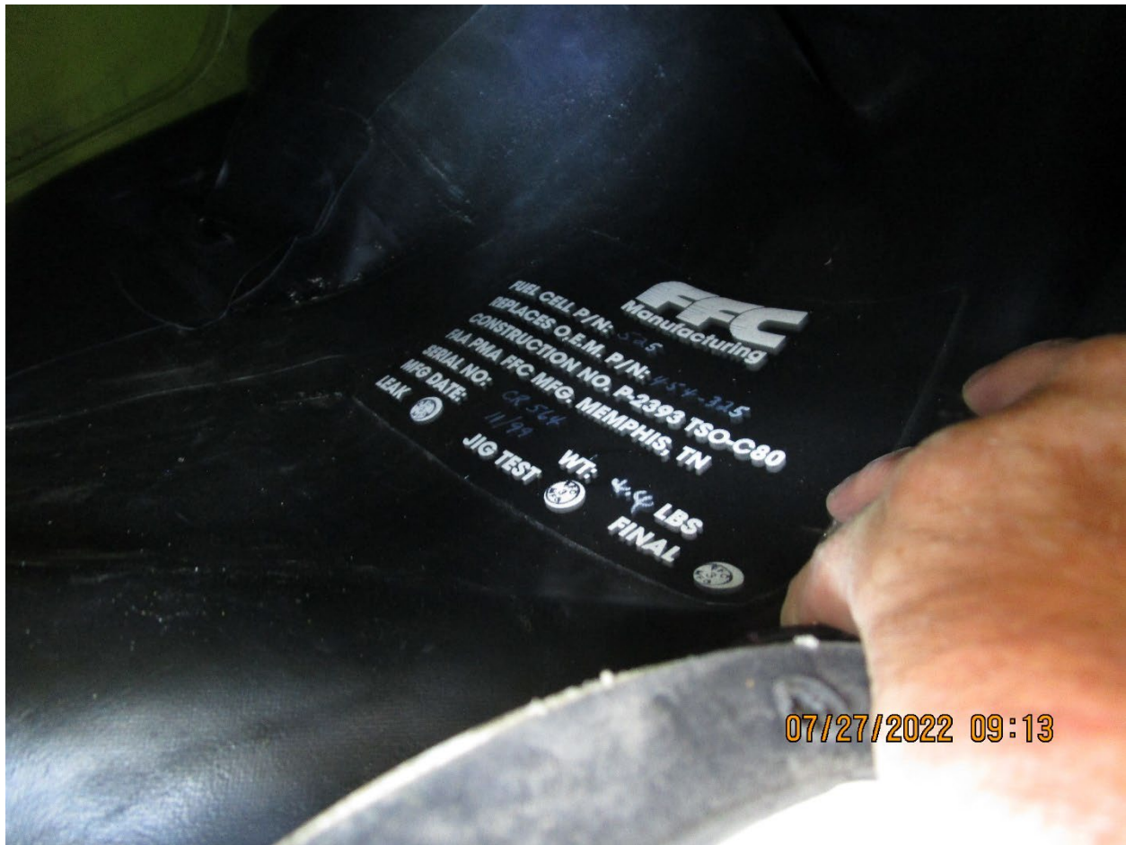
Photo 5: Right Fuel Bladder (Source - Federal Aviation Administration)
