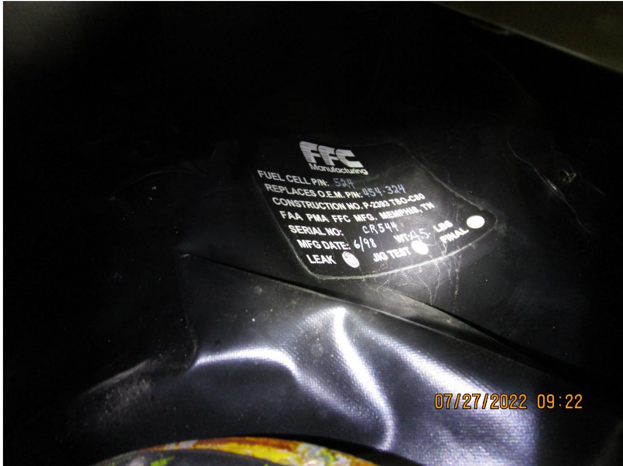
Photo 4: Left Fuel Bladder (Source - Federal Aviation Administration)
