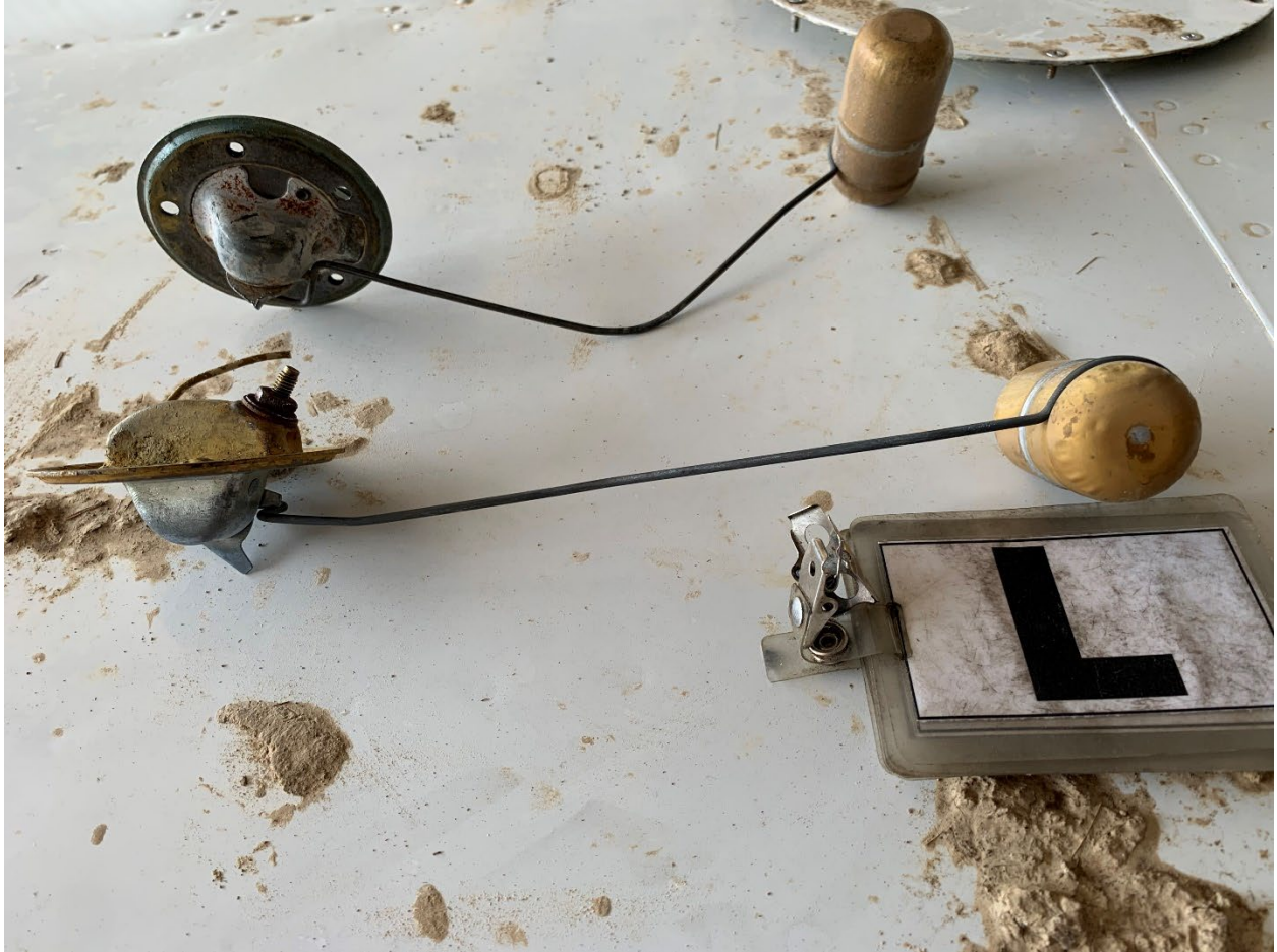
Photo 6: Left (bottom) and Right (top) Fuel Senders (Source – NTSB ICC)
