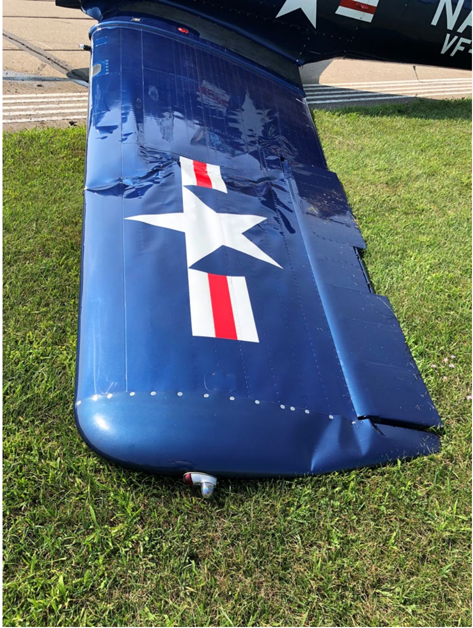
Photo 2: Left Wing Damage
