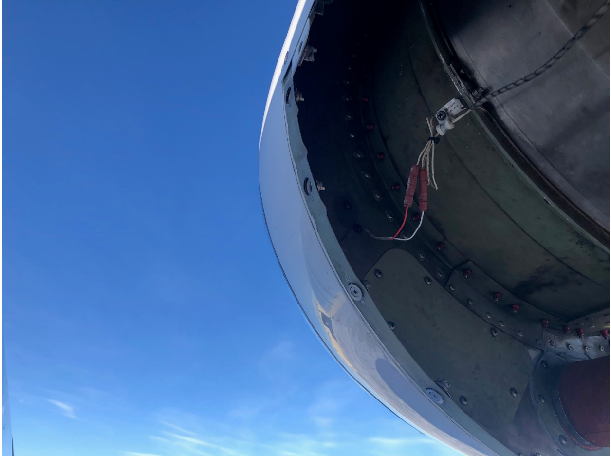
Photo 2: View of Right Engine Inboard Lower Cowl with Three Missing Fasteners
