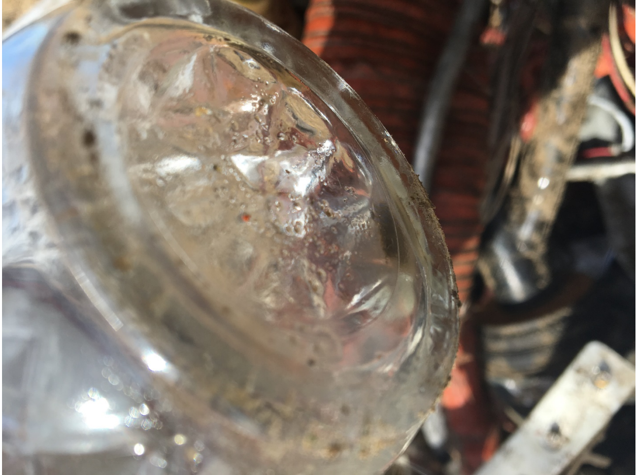
Photo 5: Fuel Sample from Fuel Line to Left Engine Fuel Manifold Valve
