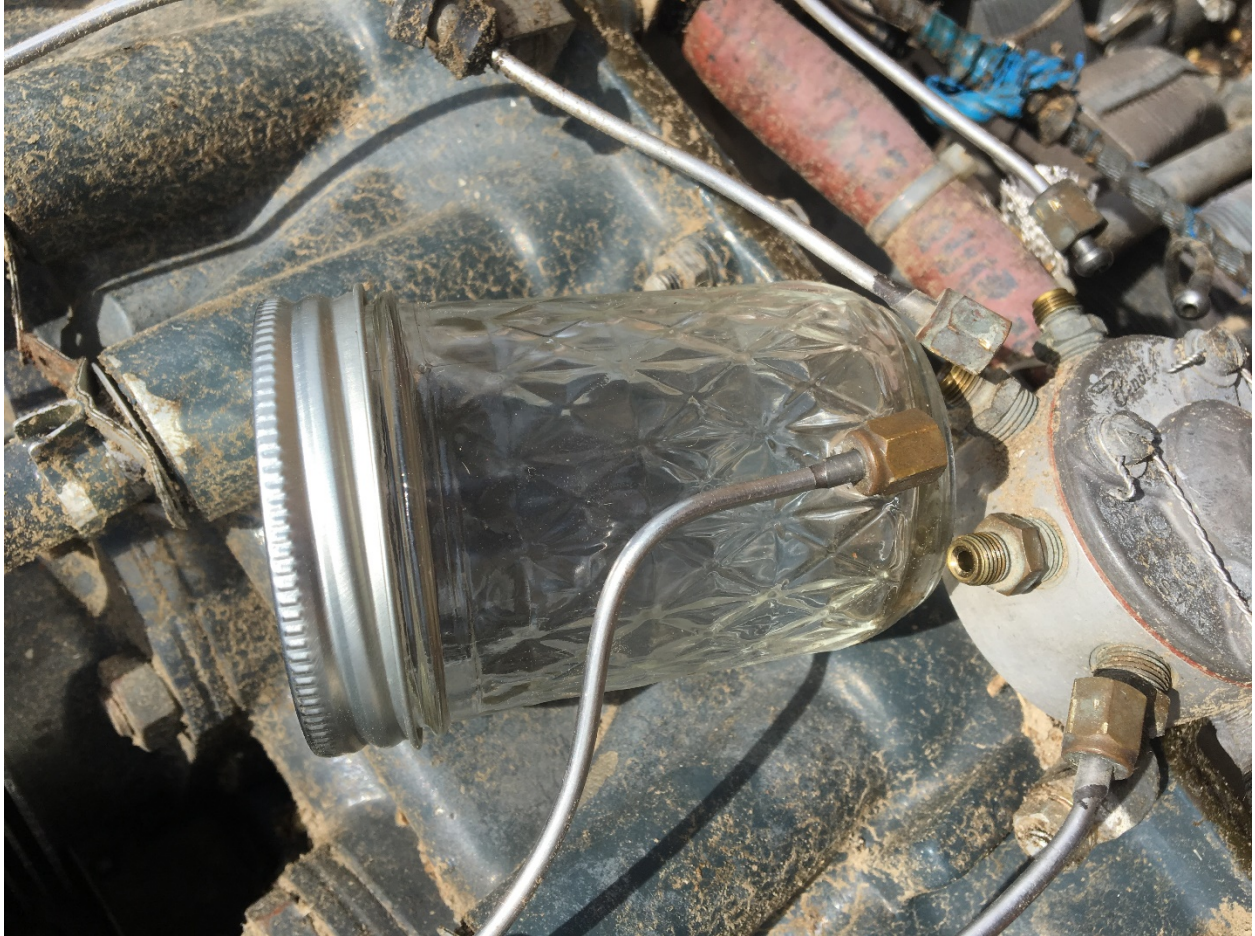
Photo 4: Fuel Sample from Fuel Line to Right Engine Fuel Manifold Valve
