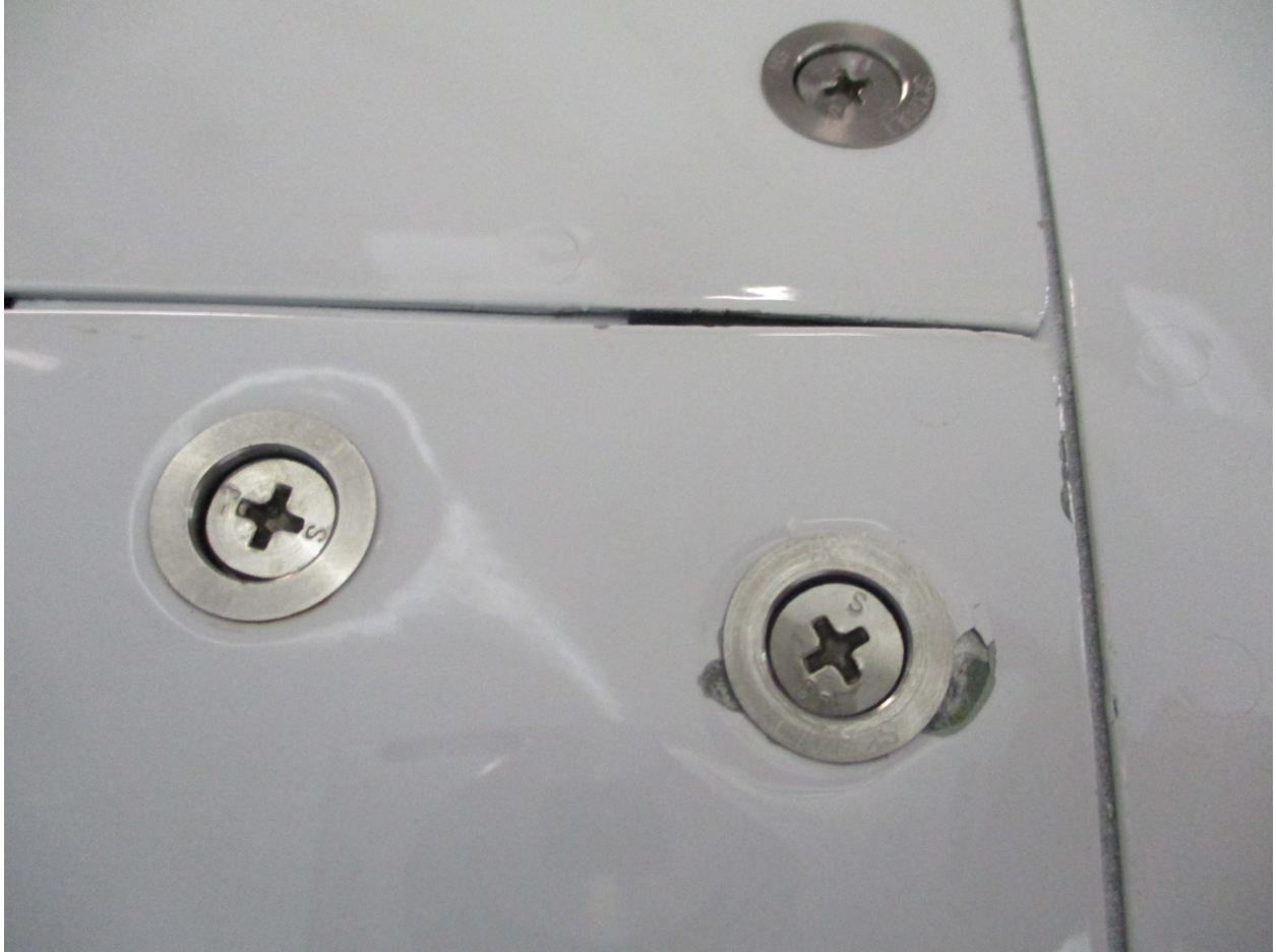
Photo 4: Fastener Assemblies of Left Engine Lower Cowl Similar to Receptacle Locations 10 and 11.
