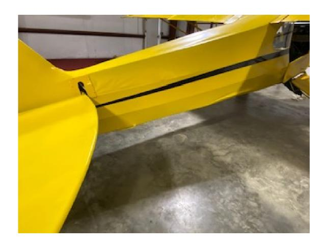
Photo 2 – Right Side Internal Structural Damage to Airframe. (Courtesy of Instructor Pilot)
