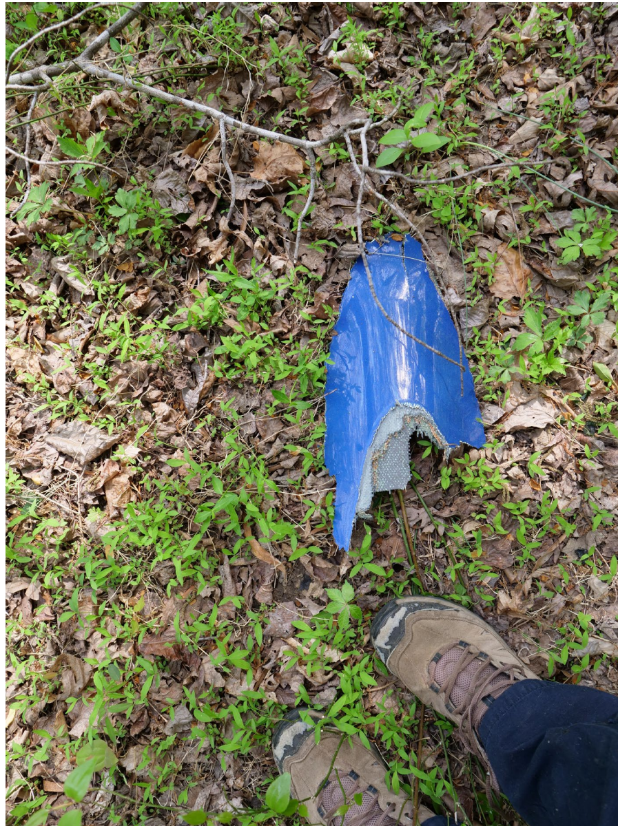
Photo 10: Damaged upper tail boom section discovered away from main wreckage. Note, this section is installed on the upper surface of the tail boom.
