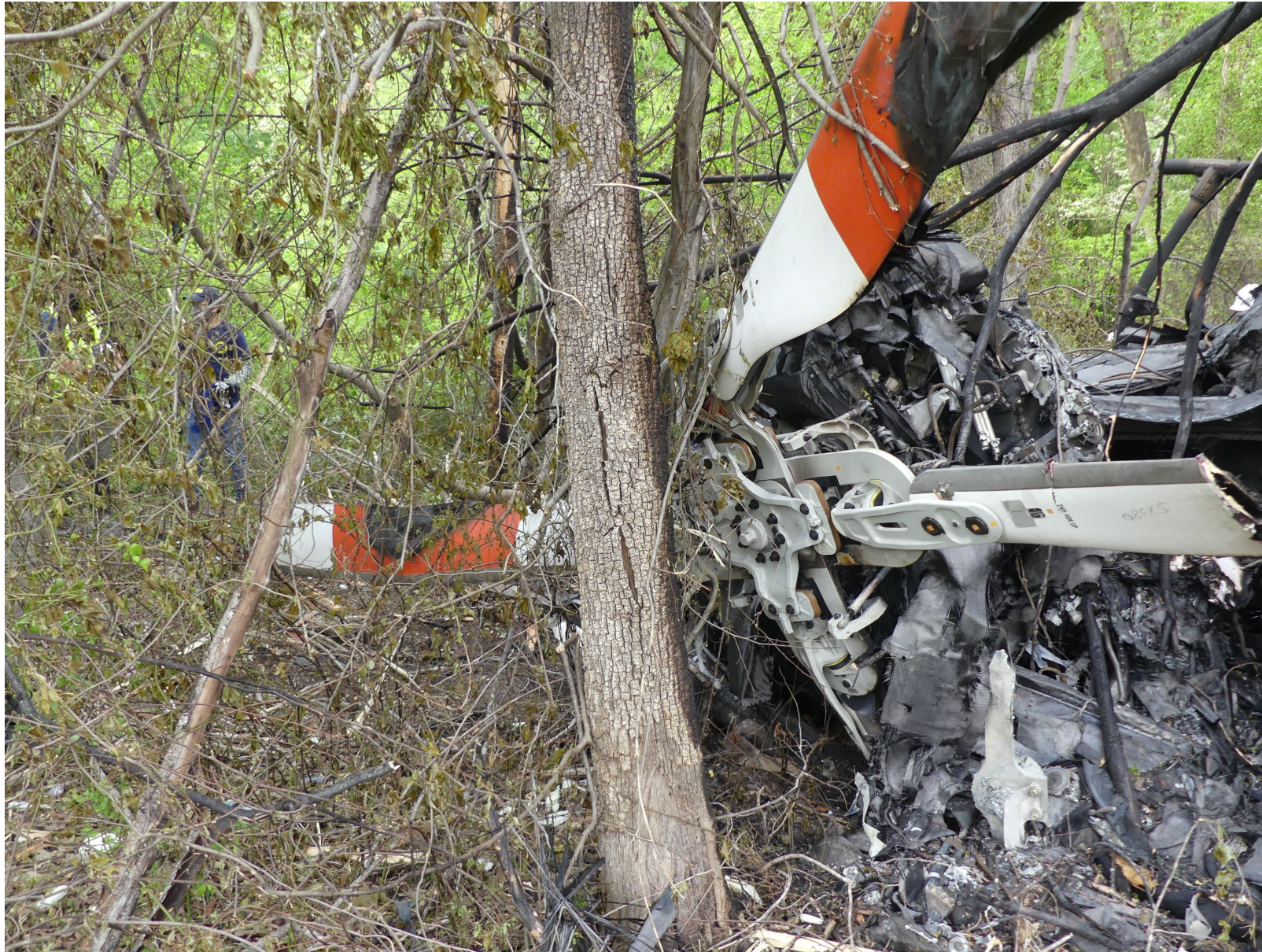
Photo 4: Closeup view of main rotor blade assembly resting up against tree.
