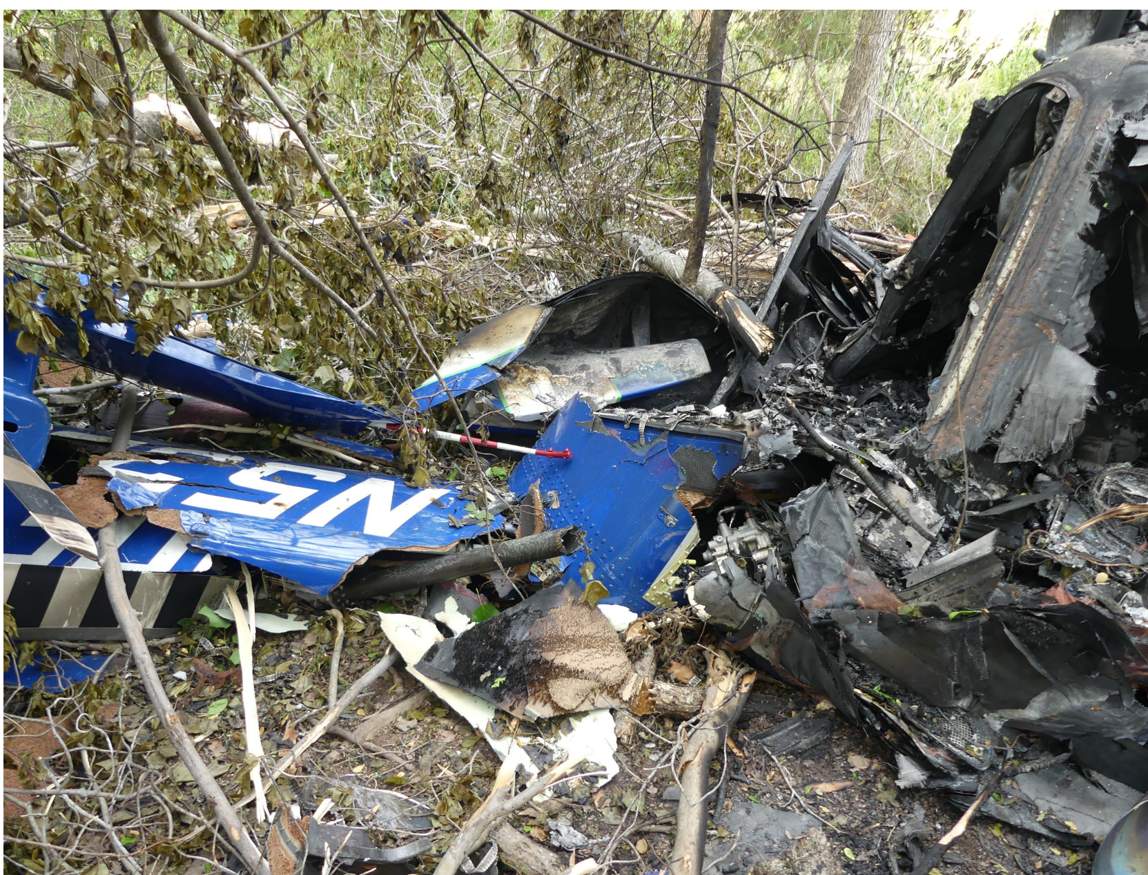
Photo 7: Tail boom on left and fuselage wreckage on right. Note tail rotor driveshaft sticking out of wreckage.
