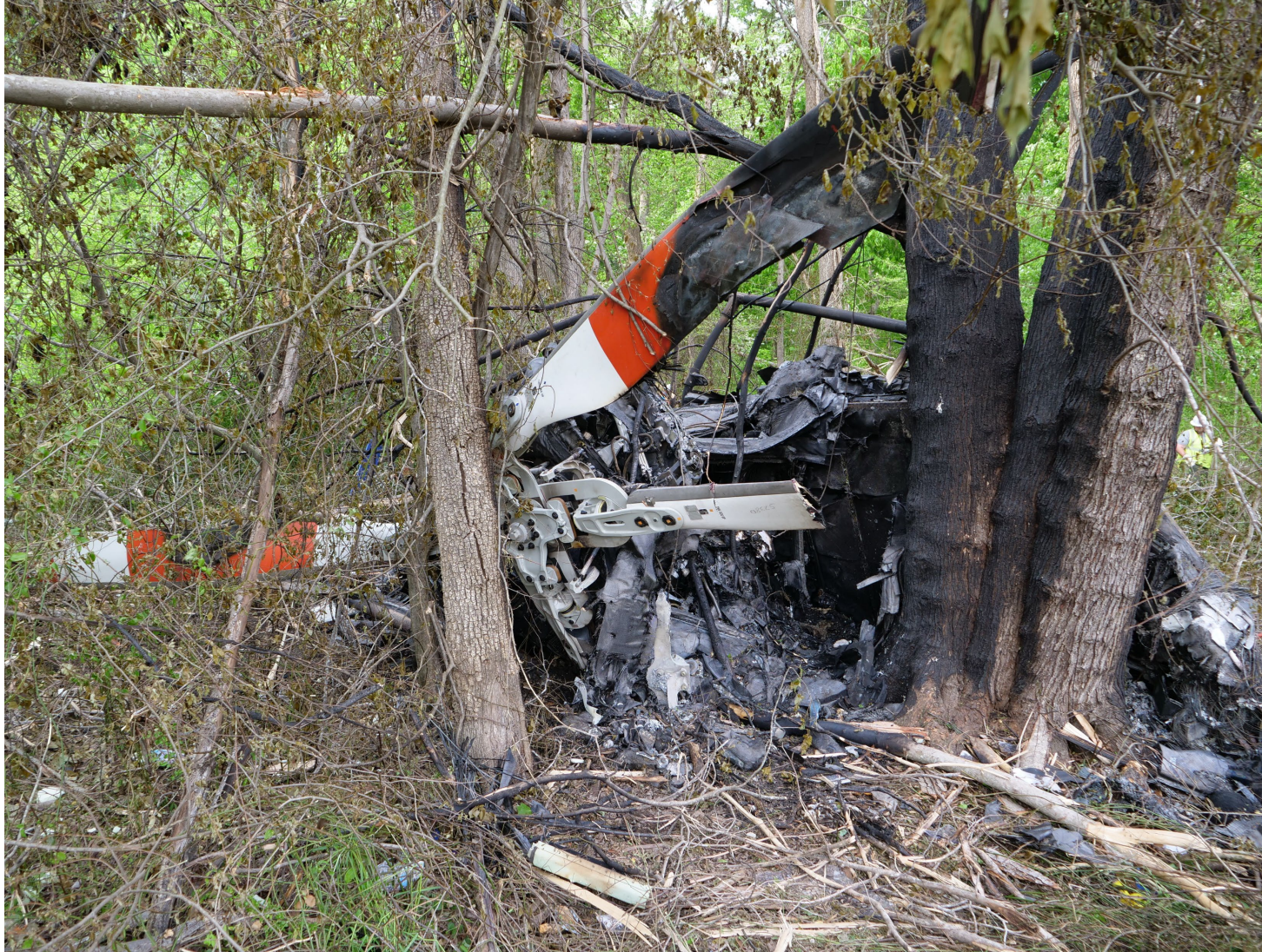
Photo 2: Main wreckage resting up against tree. Main rotor head and blades facing camera.
