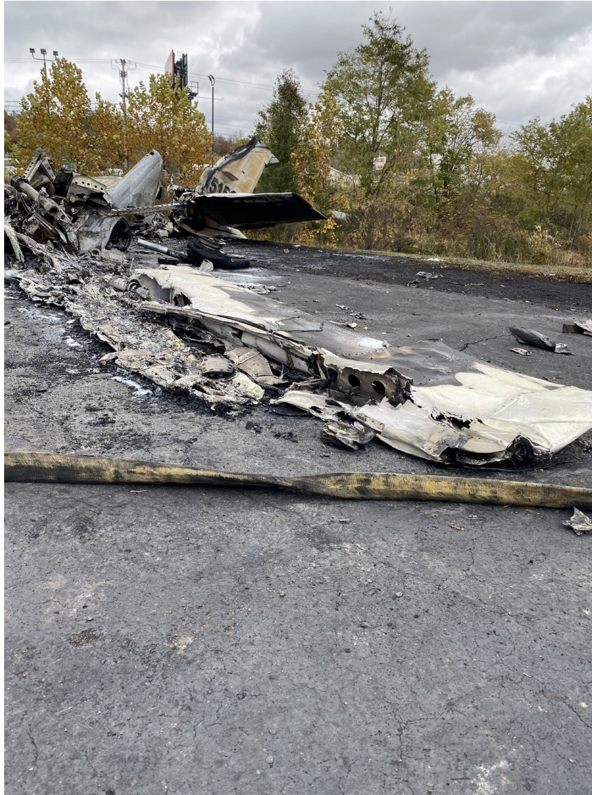
Photograph 6 - View of left wing damage.
