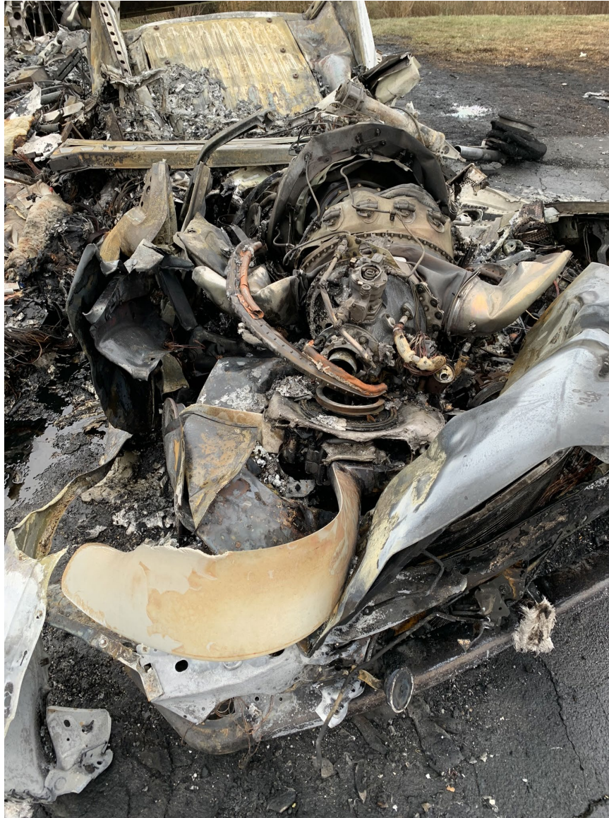
Photograph 5 - View of left propeller and engine looking aft. Note: Resting on top of damaged vehicle.
