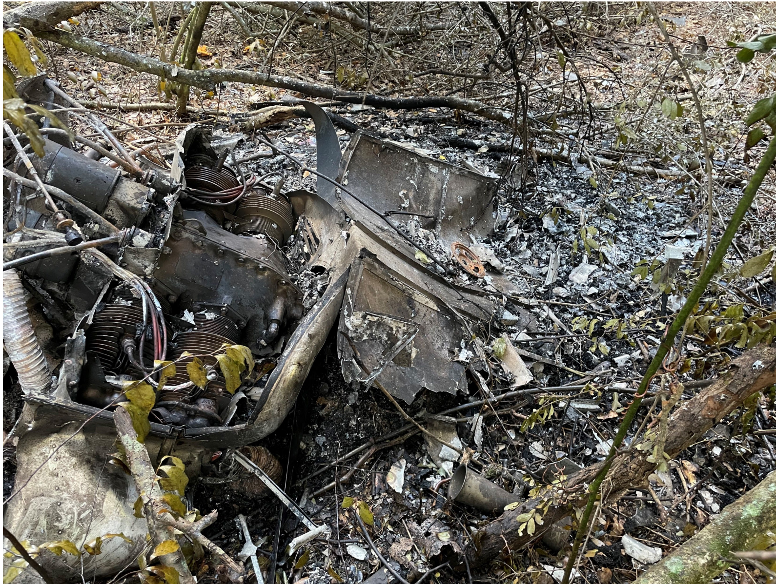
Photo 3: View of damaged engine at the wreckage site. Note thermal damage to engine. (Courtesy of FAA)
