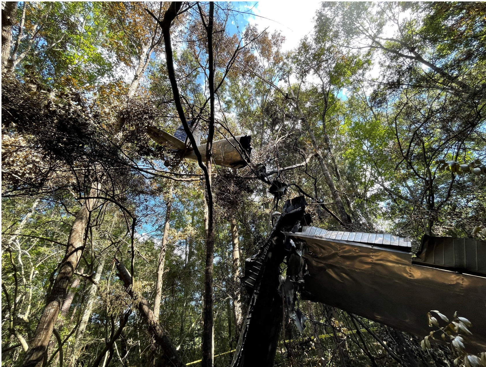
Photo 4: Wide angle view of empennage stuck up in trees. (Courtesy of FAA)
