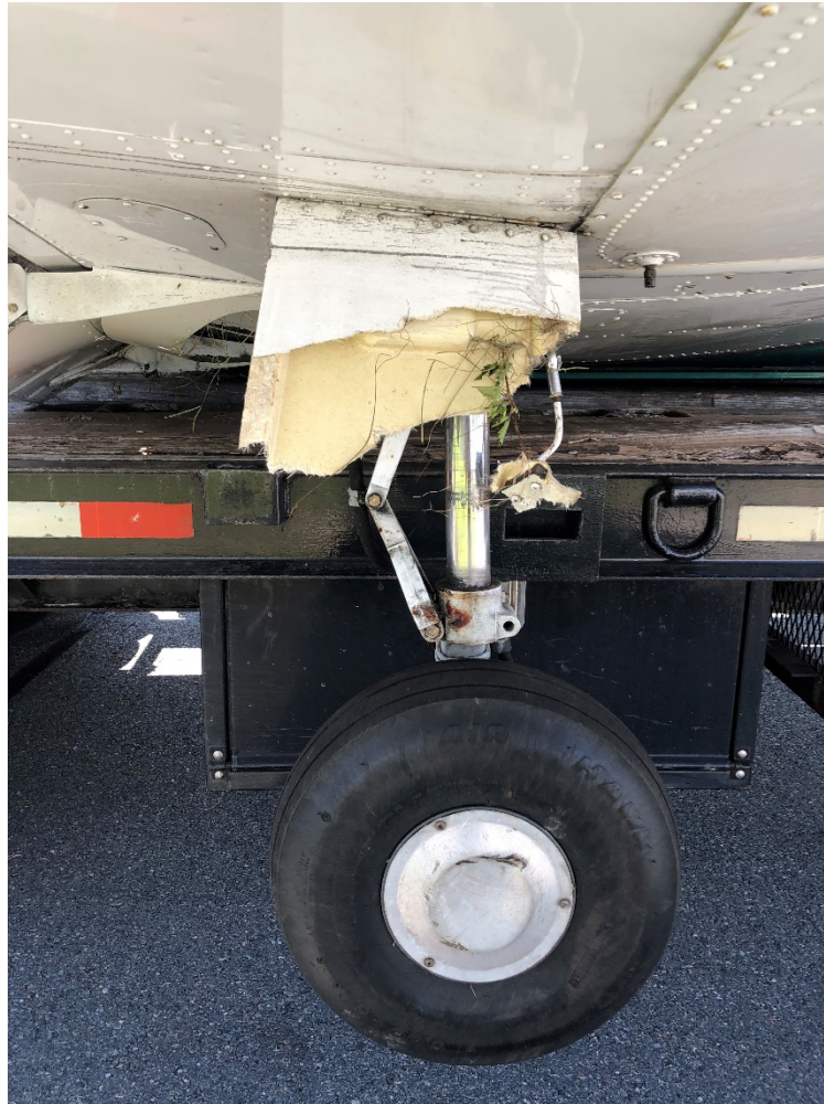
Photo 6 – View of the left main landing gear (Photo Courtesy of FAA)
