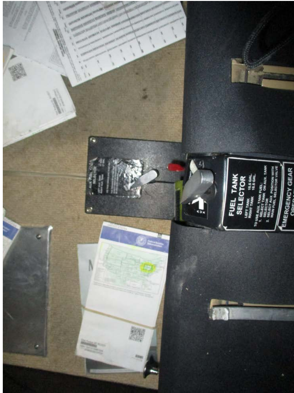
Photo 6 – Fuel Selector (FAA Photo)
