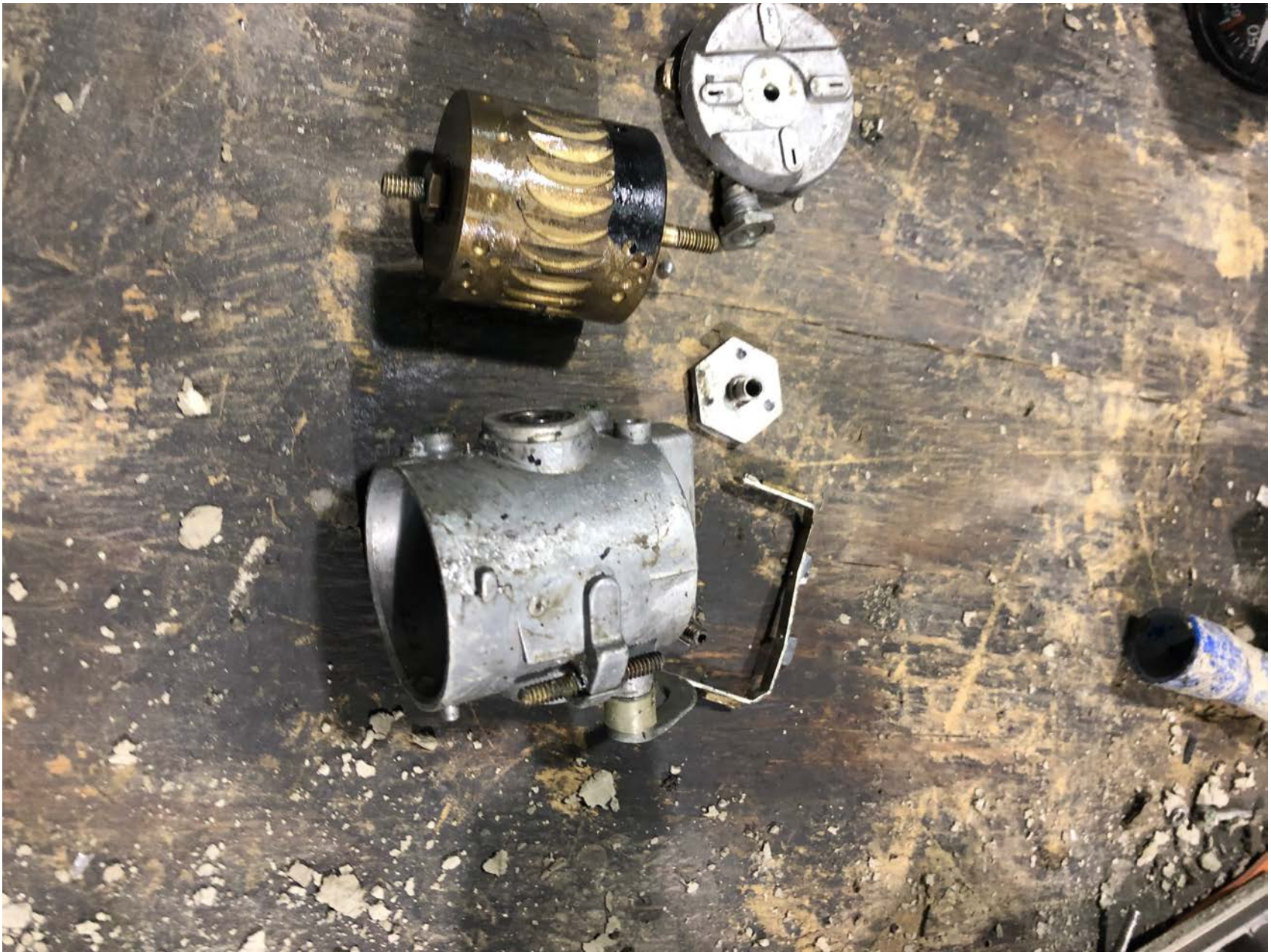
Photo 4 - Attitude indicator gyro and gimble.
