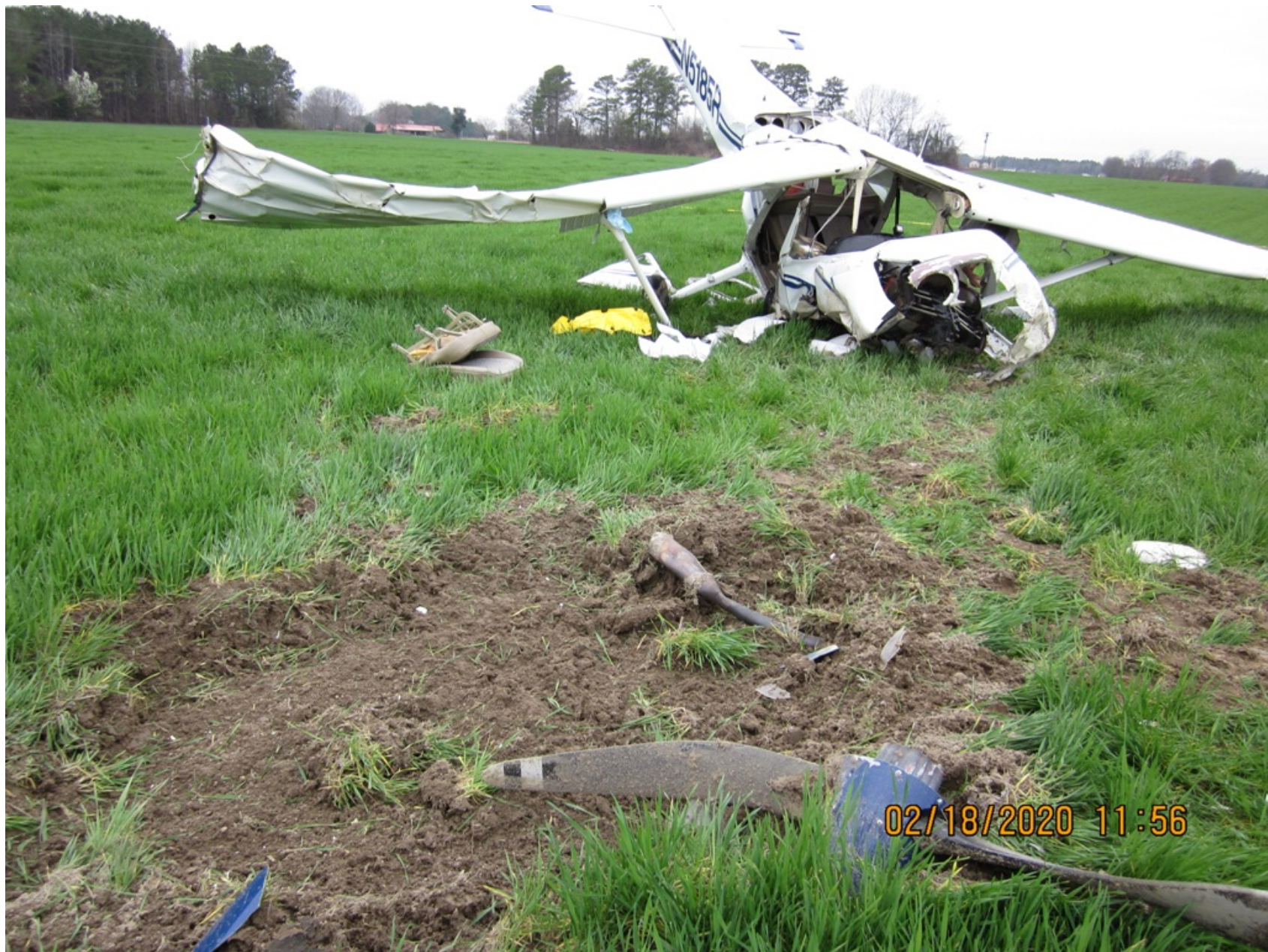
Photo 3 - Main Wreckage and Point of Initial Ground Impact (FAA Photo)
