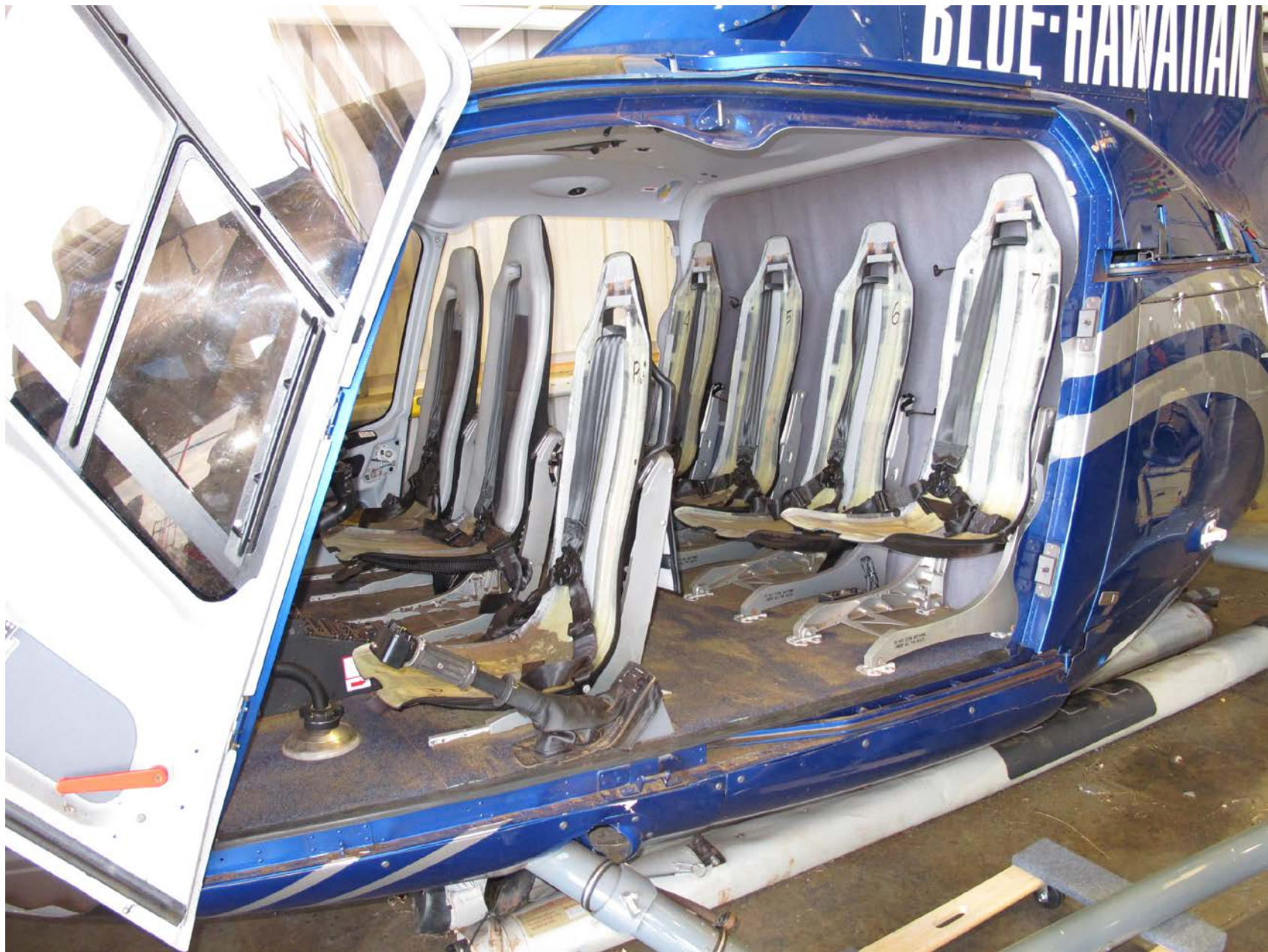
Photo 10 – View of the helicopter cabin showing all 7 seats after the accident. Seat cushion material removed.
