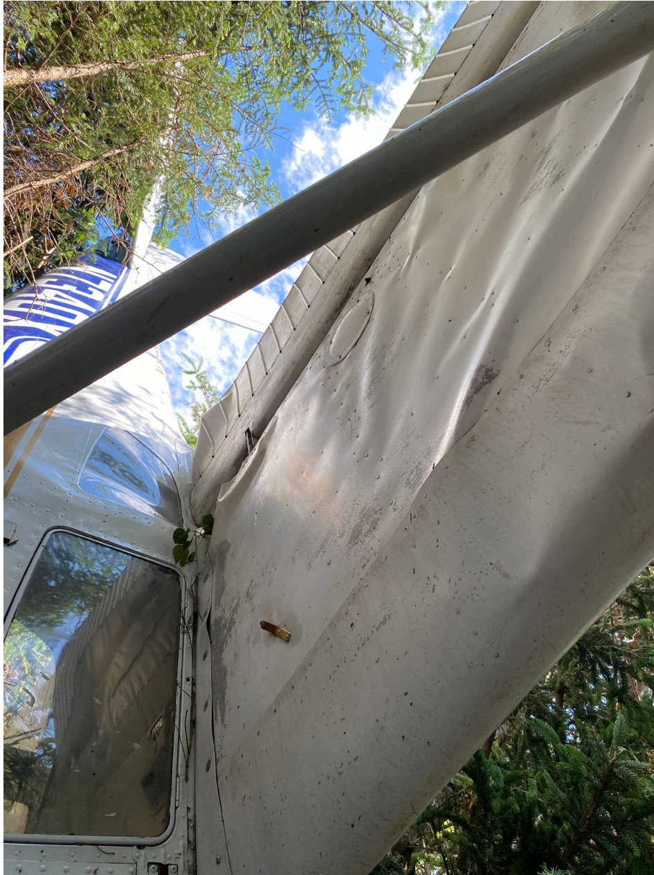
Photo 2 – View of Damage to Right Wing (FAA)
