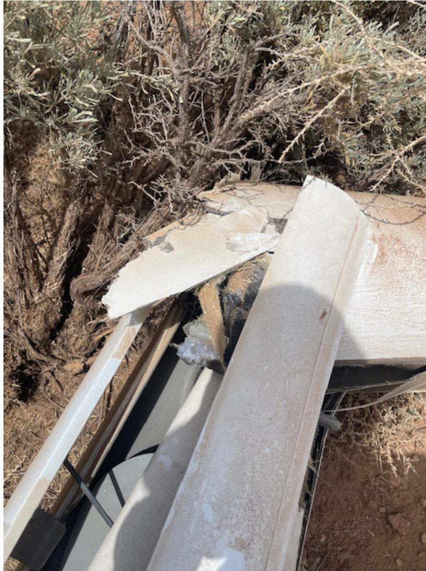
Photograph 3 - View of damage to empennage. (Courtesy of Iron County Sheriff's Dept.)
