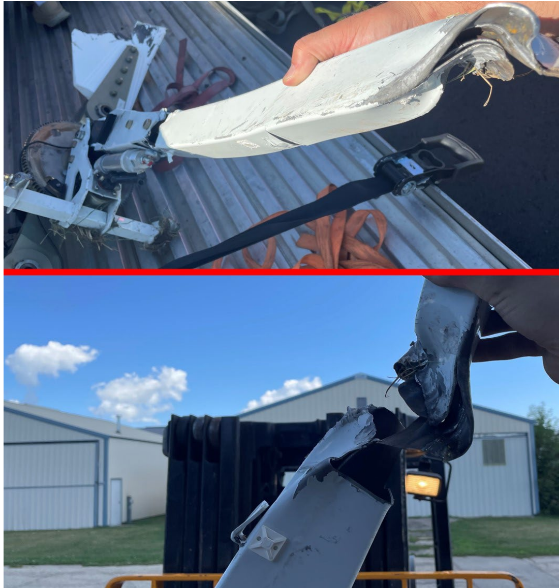
Photograph 5 - Gyroplane's separated rotor mast
