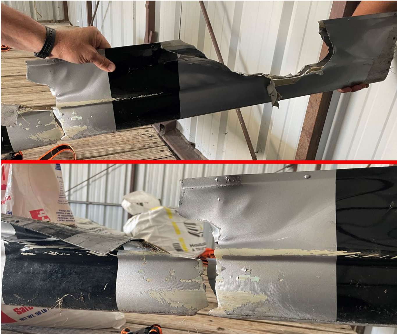
Photograph 3 - Separated outboard sections of the helicopter main rotor blades
