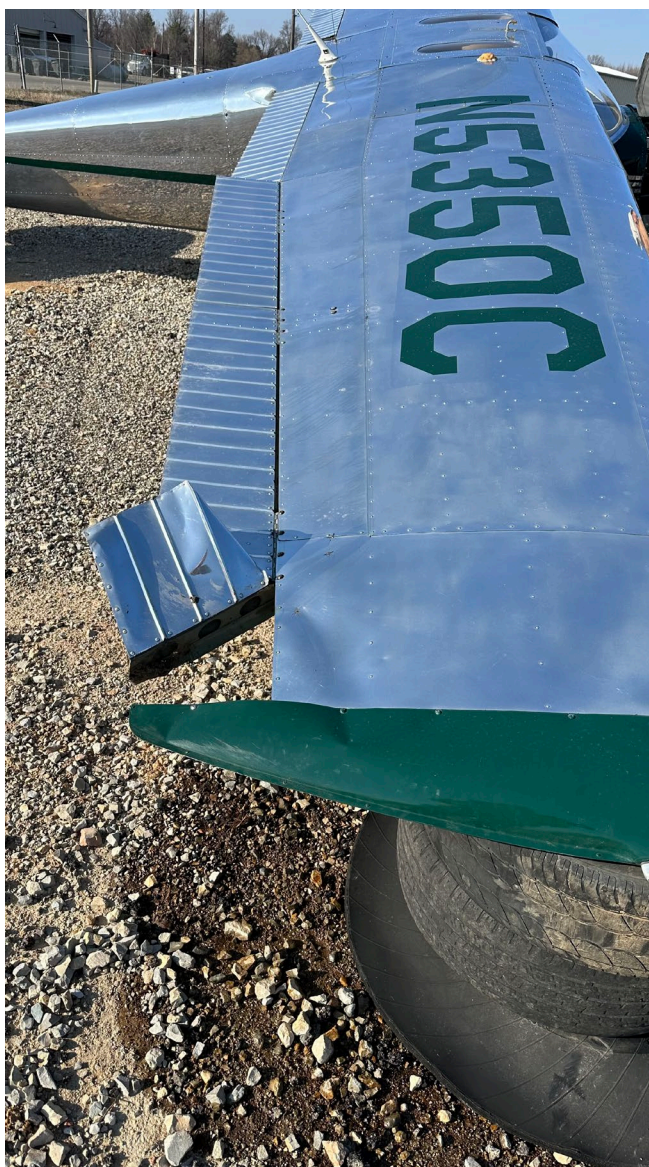
Photograph 2 - Deformation noted to the right aileron (Courtesy of Pilot)
