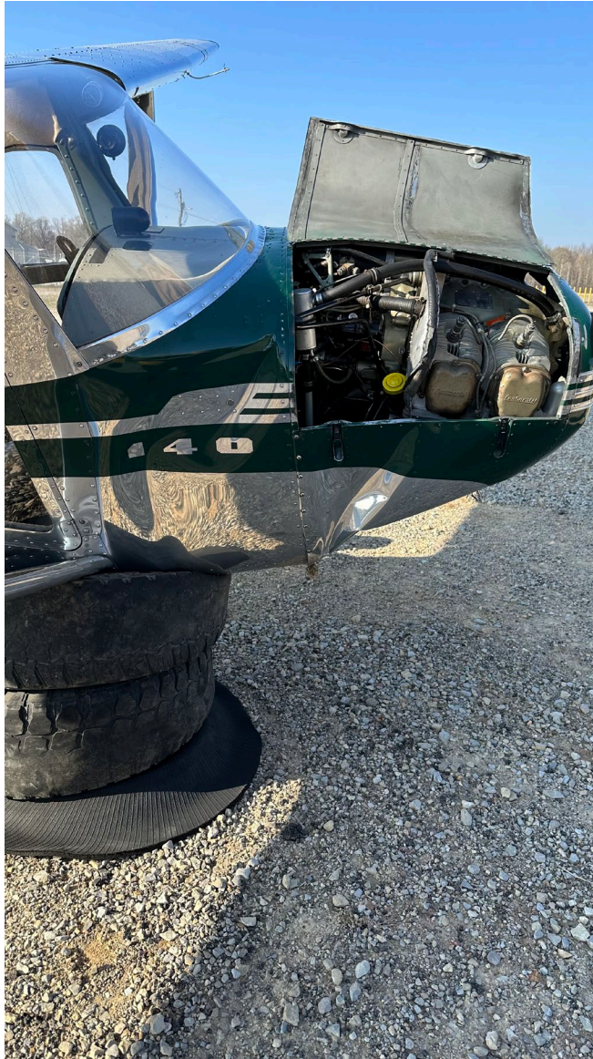
Photograph 3 - Deformation noted to the fuselage (Courtesy of Pilot)
