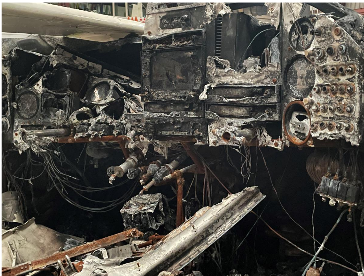
Photograph 2 - Burned Airplane Instrument Panel (Courtesy of FAA)
