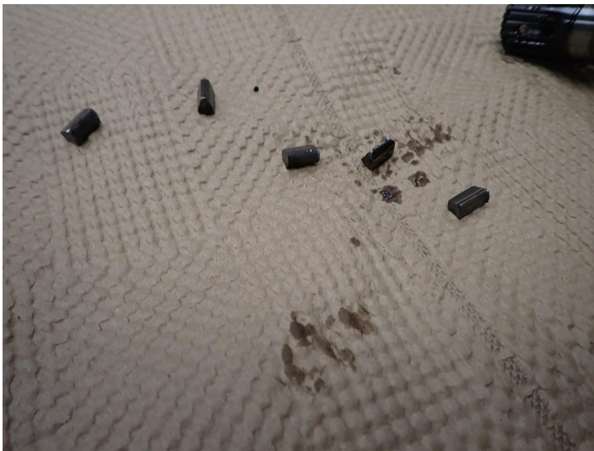
Photograph 4 - Camshaft Teeth Found in Oil Sump
