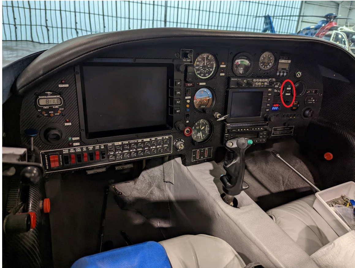
Photograph - Turbocharger Switch in Cockpit (Courtesy of Owner)
