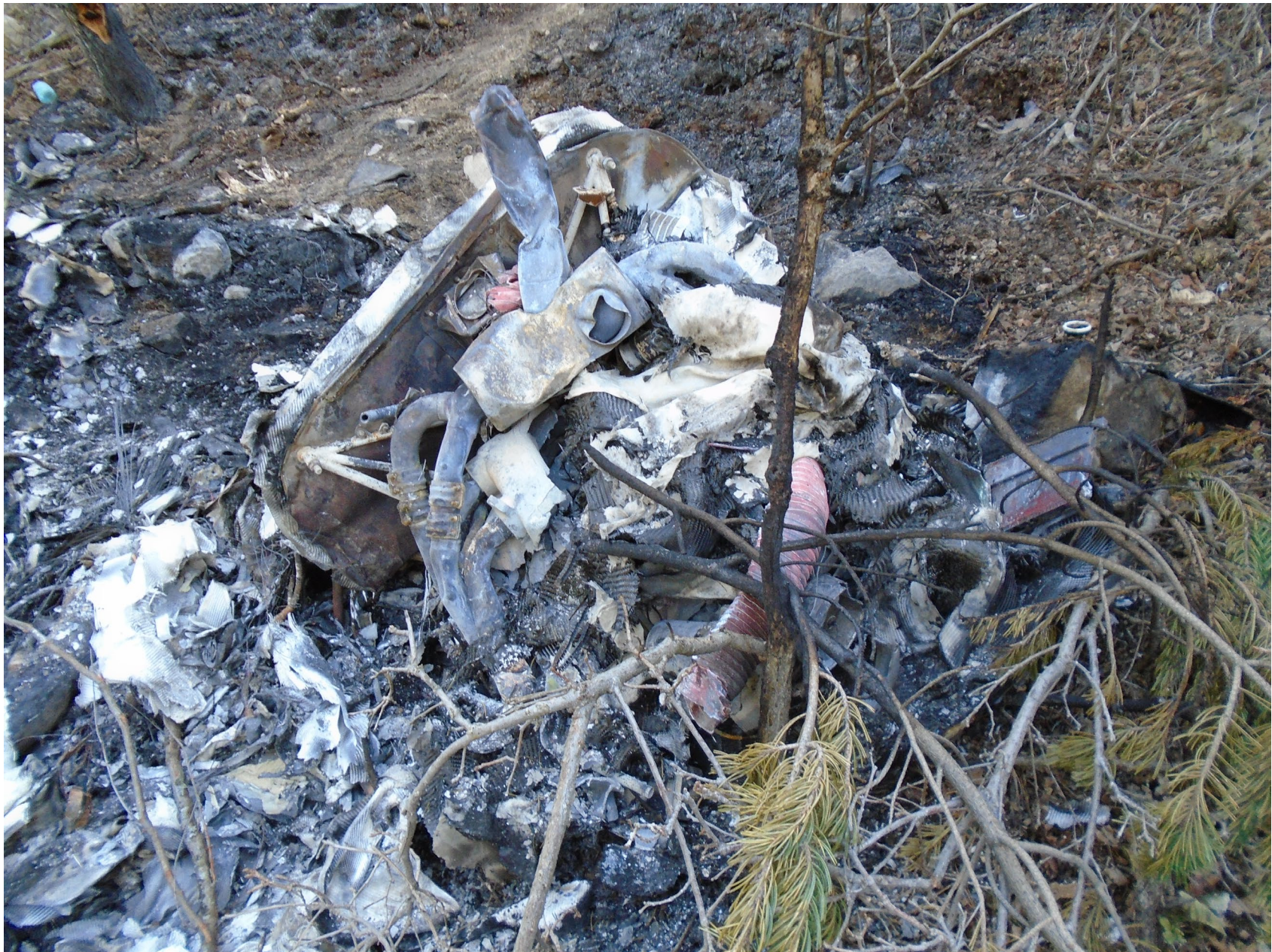
Photo 1 – View of thermal damage to airplane firewall
