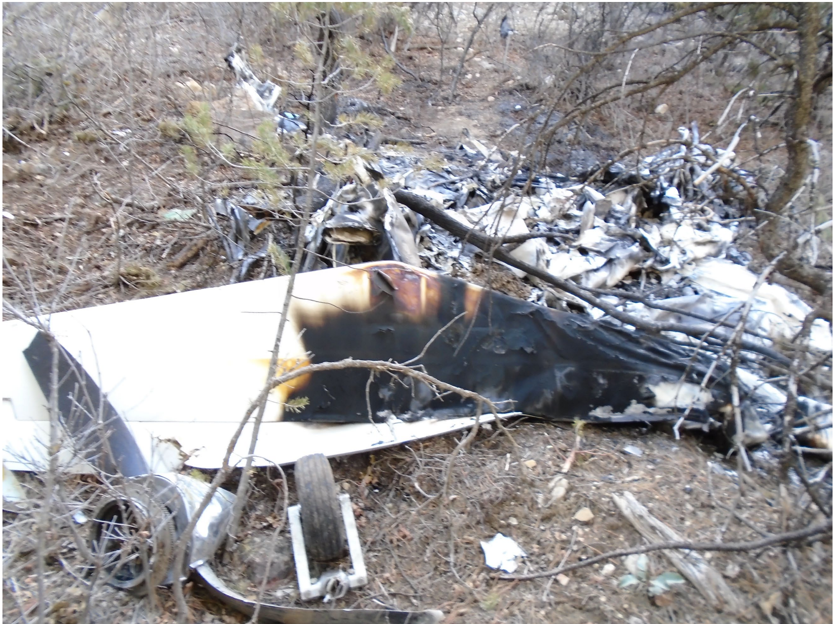
Photo 4 – View of thermal damage to airplane horizontal stabilizer
