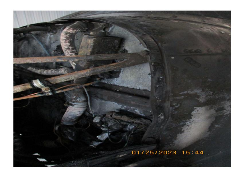
Photo 4 – View of fire damaged engine mounts and firewall (Photo courtesy of FAA)
