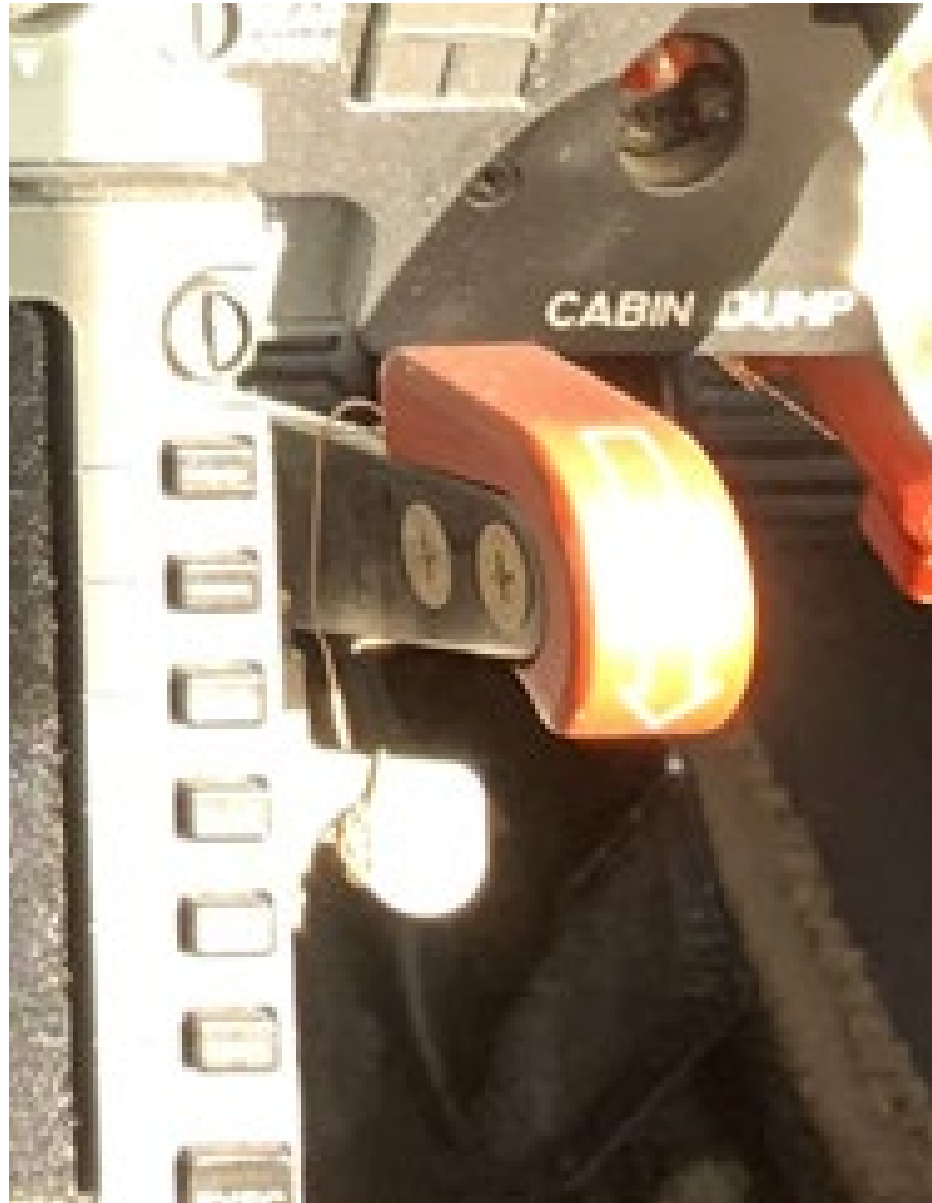
Photo 7 – Emergency Brake Control Lever
