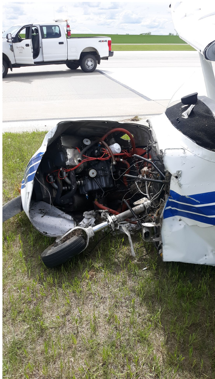
Photo 2 – Engine damage – Courtesy of FAA
