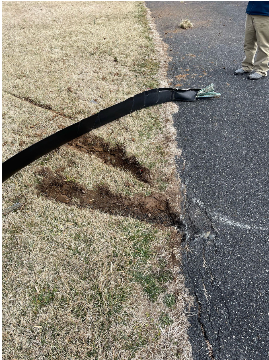
Photo 3 – Ground Scar from Main Rotor – Courtesy of FAA
