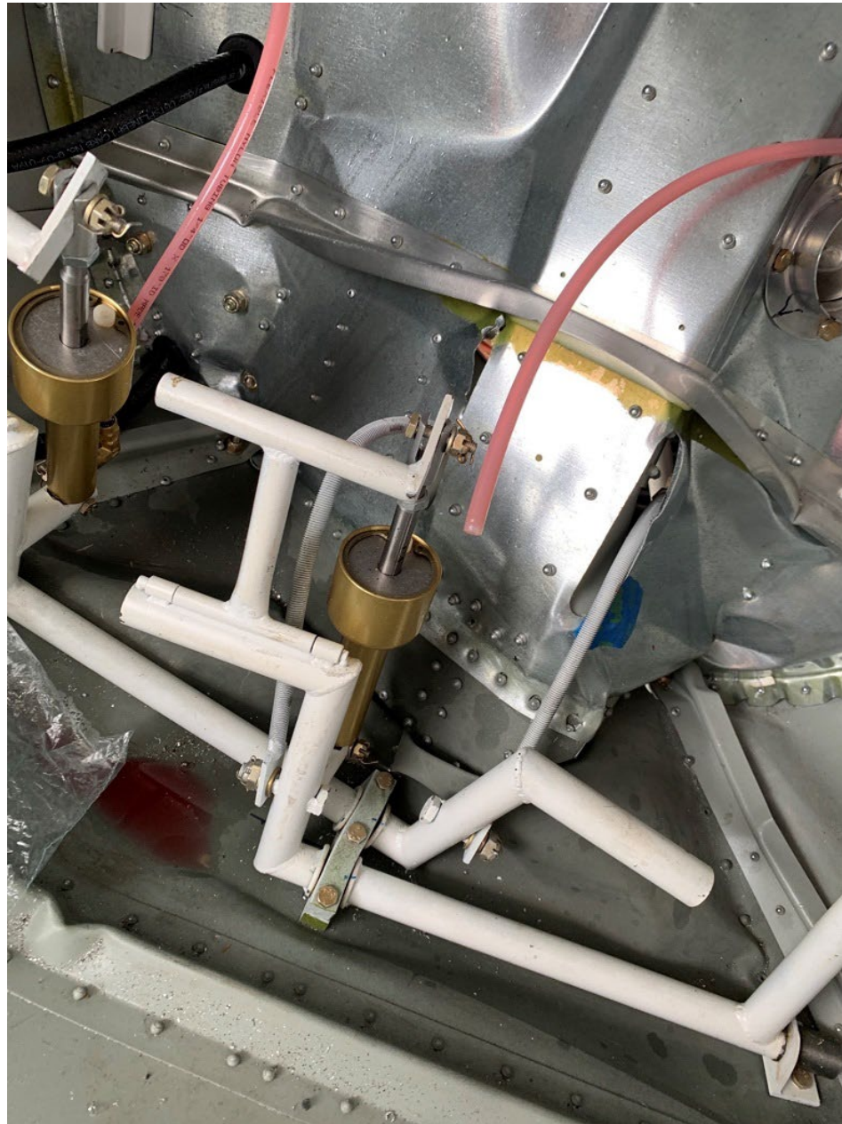
Photo 2 – Lower Fuselage Damage (Photo Courtesy of FAA)
