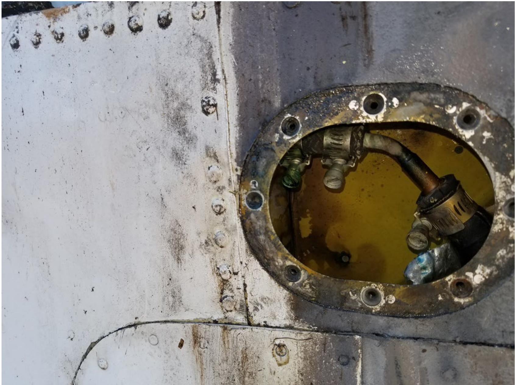
Photo 2 - Loose Aux Fuel Tank Fitting in RH Wing (FAA)
