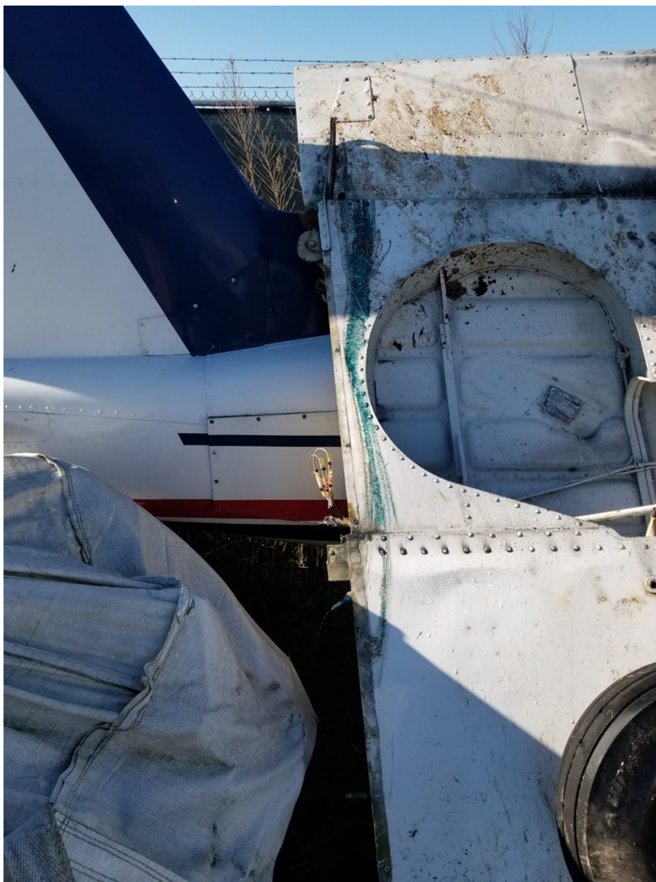
Photo 3 – Fuel Stain at Root of RH Wing (FAA)
