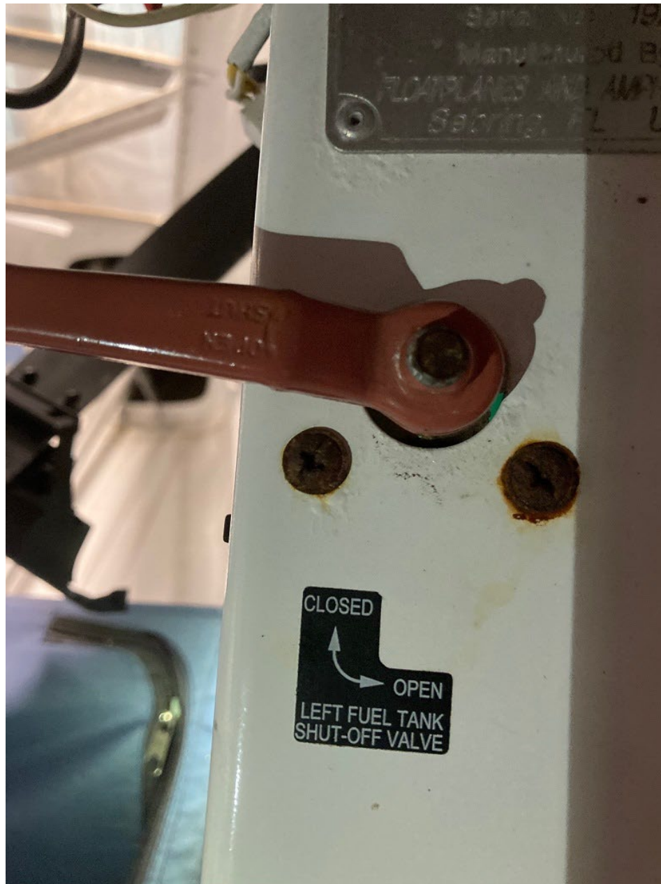
Photo 3 – Left Wing Tank Fuel Valve (Photo Courtesy of Pilot)
