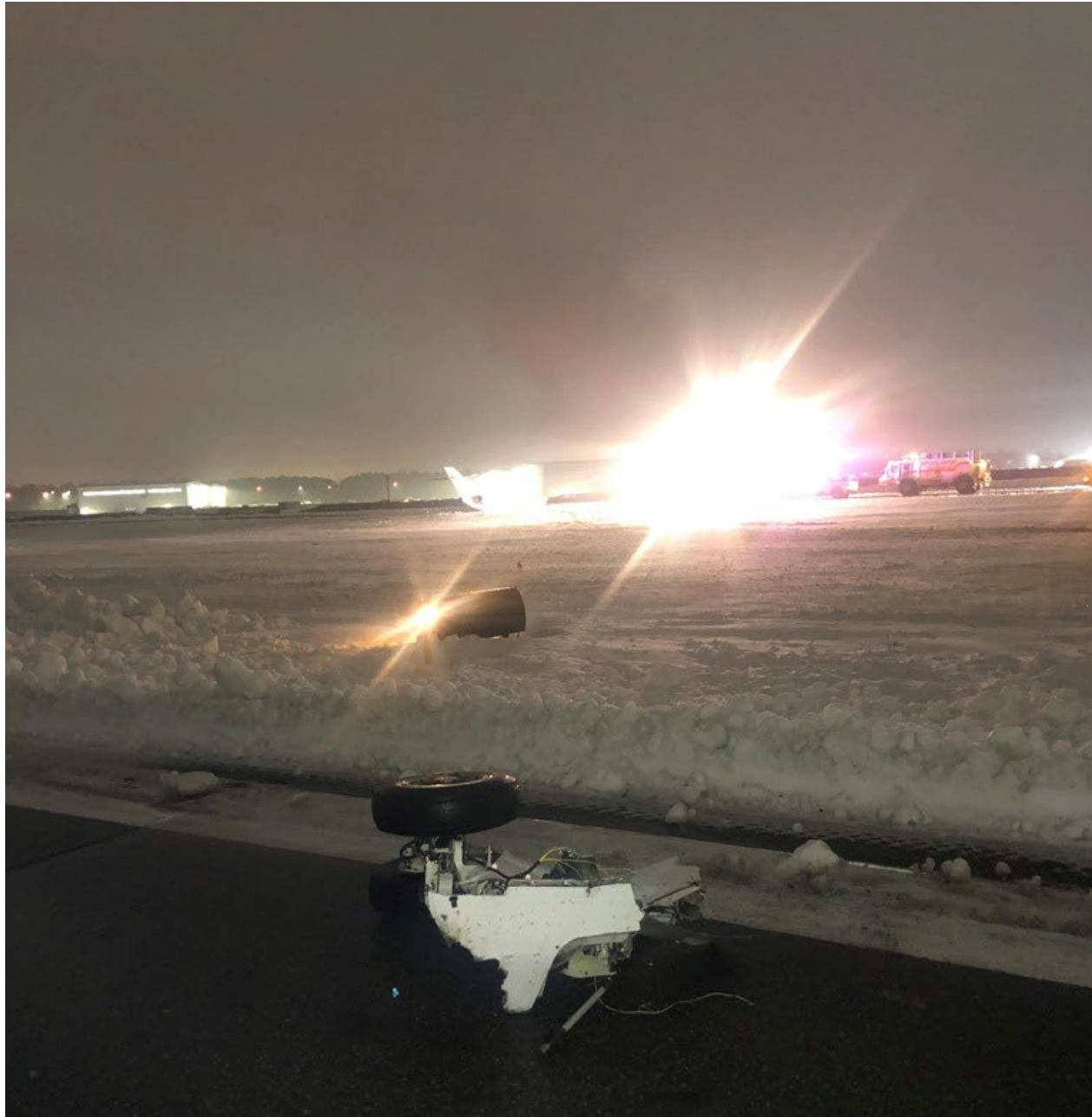
Photo 2 – Section of Landing Gear on Runway with Airplane in the Background (FAA)
